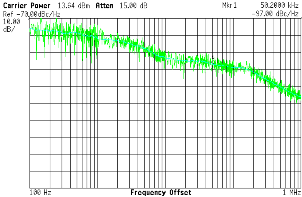
Figure 29. Typical SX1230 Phase Noise Measured at 868 MHz (-97 dBc/Hz at 50 kHz).
