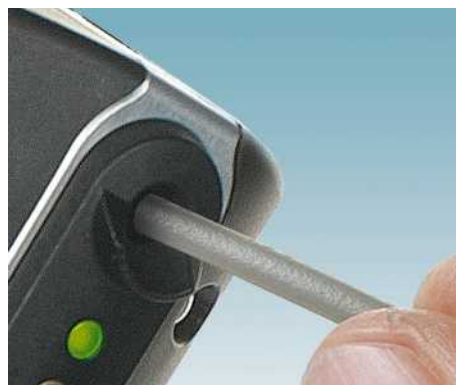
... stripping and crimping is carried out automatically, ...
