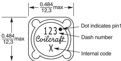
Parts manufactured prior to Sept. 2007 were marked with only the dash number.
