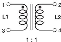
Tight coupling ( $k \geq 0.98$ ) and 500 V isolation make the MSD1278 series of shielded coupled inductors ideal for use in a variety of circuits including flyback, multi-output buck and SEPIC.
