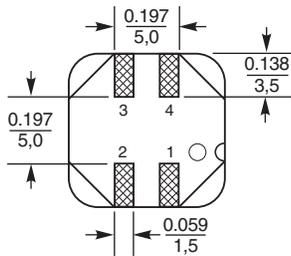
\* For optional tin-lead and tin-silver-copper terminations, dimensions are for the mounted part. Dimensions before mounting can be an additional 0.012 inch (0,3 mm).
