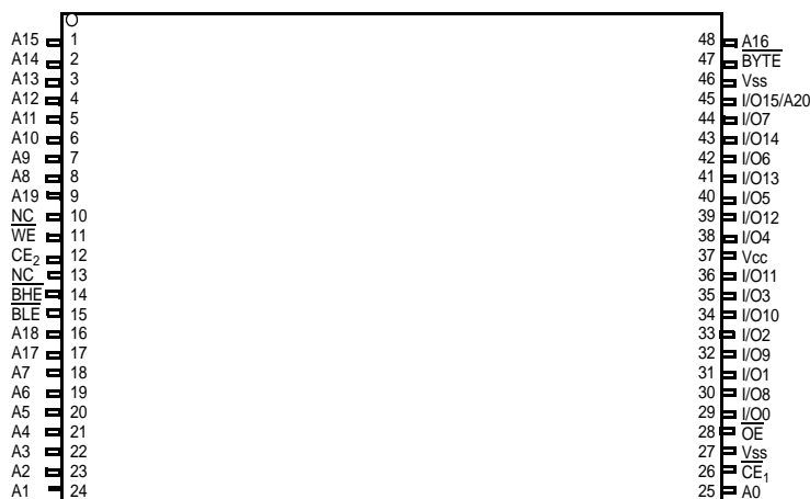
Figure 2. 48-pin TSOP I (12 × 18.4 × 1.0 mm) Top View [2, 3]
