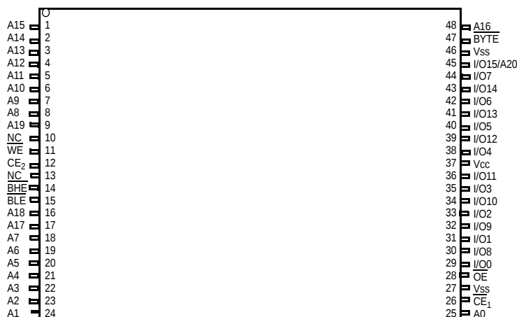
Figure 2. 48-pin TSOP I (12 × 18.4 × 1.0 mm) Top View [2, 3]
