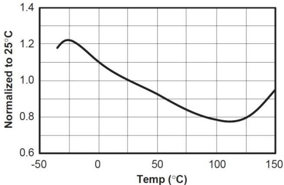
Figure 6. Startup Current
