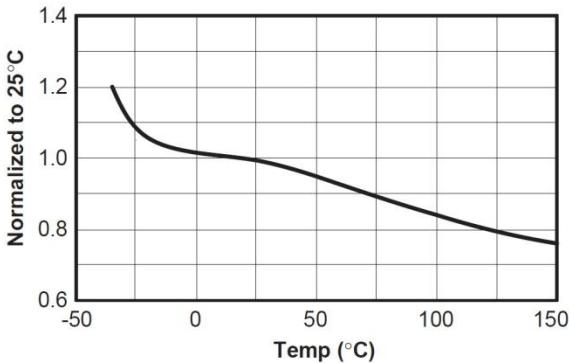
Figure 5. Burst Mode Supply Current (Non-Switching)
