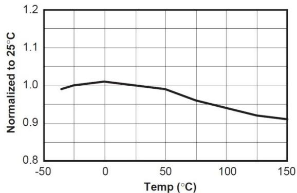
Figure 15. Burst Mode Feedback Source Current
