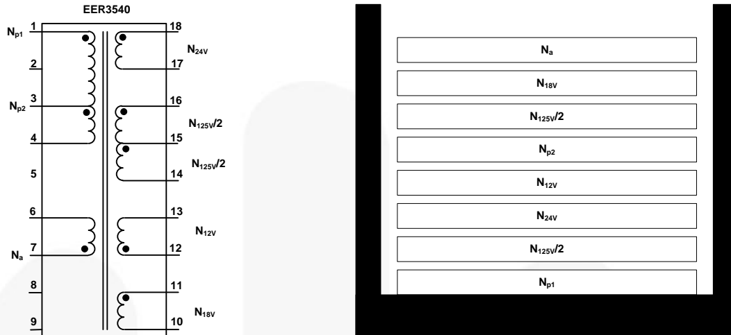
Figure 42. Transformer Schematic Diagram
