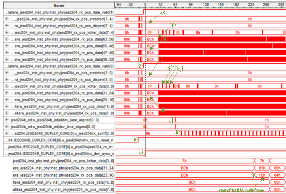
Figure 33. JESD204B Link Initialization
