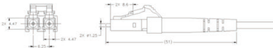
LC Duplex Connector with 1.6/2.0mm Boots
