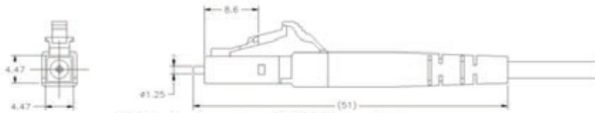
LC Simplex Connector with 1.6/2.0mm Boot
