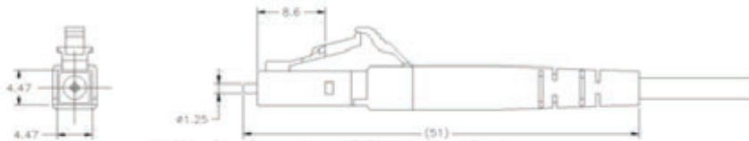
LC Simplex Connector with 1.6/2.0mm Boot
