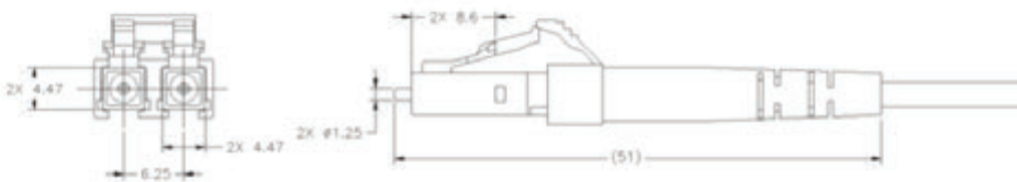
LC Duplex Connector with 1.6/2.0mm Boots
