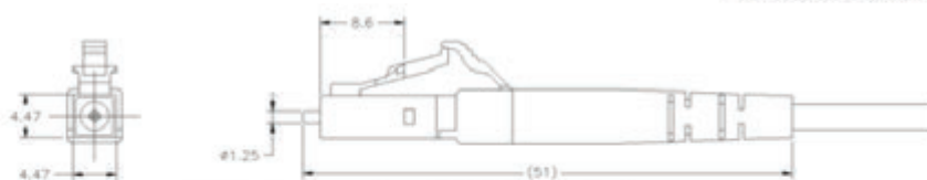
LC Simplex Connector with 1.6/2.0mm Boot
