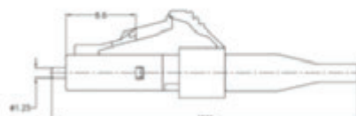
LC Duplex Connector with 900μm Boot
