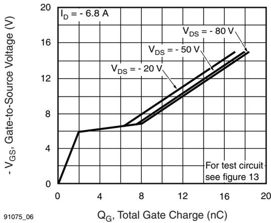
Fig. 6 - Typical Gate Charge vs. Gate-to-Source Voltage
