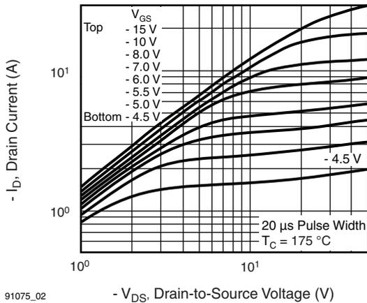
Fig. 2 - Typical Output Characteristics,  $T_C = 175\text{ }^\circ\text{C}$
