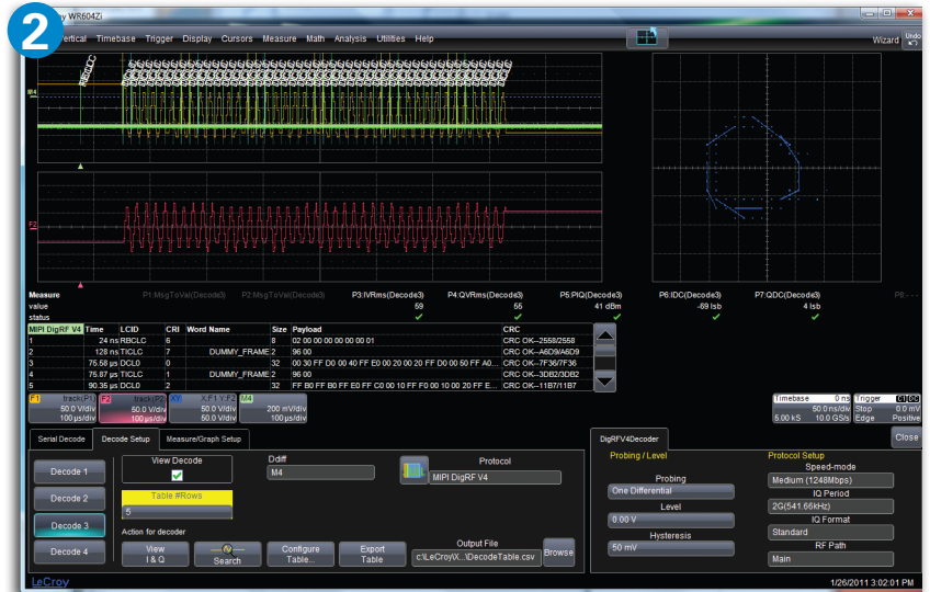
DigRF v4 Constellation diagram shows information such as gaussian noise, Phase noise, and attenuation.
