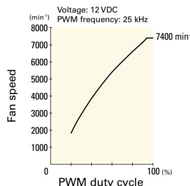
**9LG0812P4G001** With pulse sensor with PWM control function
