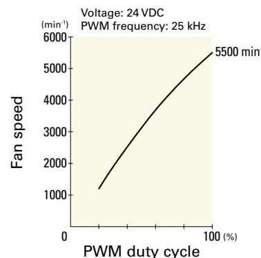
**9LG0824P4H001** With pulse sensor with PWM control function
