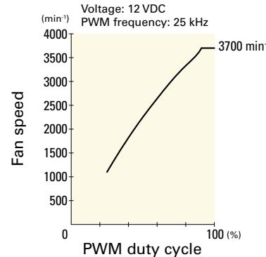
**9LG0824P4J001** With pulse sensor with PWM control function
