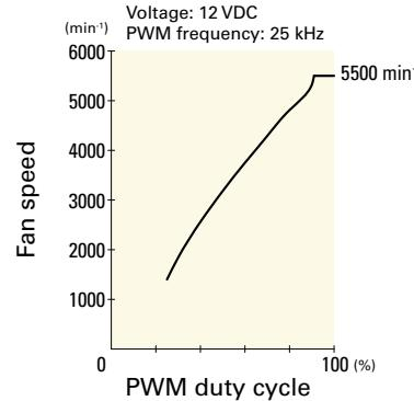
**9LG0812P4H001** With pulse sensor with PWM control function
