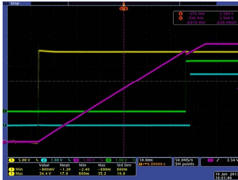
Figure 6. NCN5150 Startup Sequence
