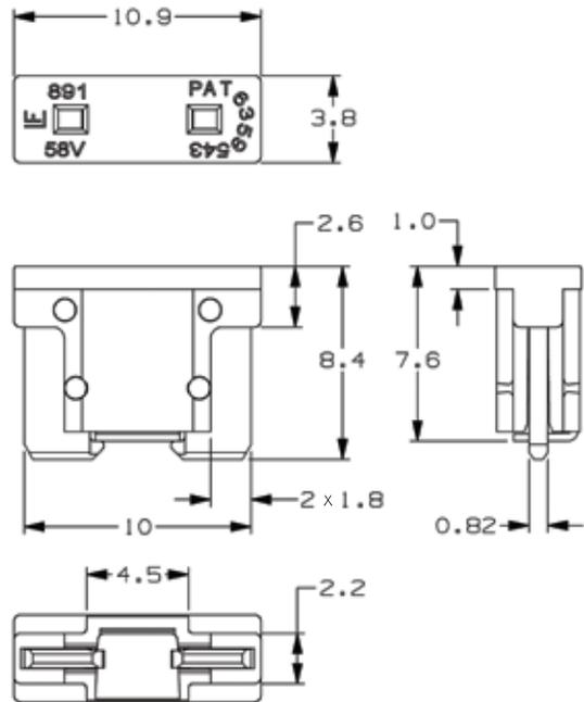
The Low Profile MINI® fuse has similar performance characteristics as the standard MINI® fuse. The lower overall height allows for more space and weight savings. The Low Profile MINI® fuse is designed to mate with tuning-fork terminals, which provides additional weight and material savings in fuse box designs by eliminating the need for female box terminals.
