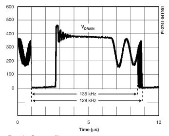
Figure 4. Frequency Jitter.
