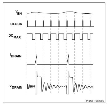
Figure 9. Operation at Very Light Load.
