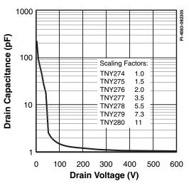
Figure 25.  $C_{\rm oss}$  vs. Drain Voltage.
