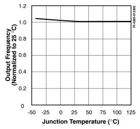
Figure 21. Frequency vs. Temperature.
