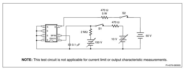
Figure 16. General Test Circuit.
