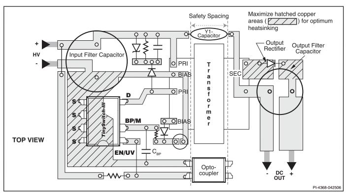
Figure 15. Recommended Circuit Board Layout for TinySwitch-III with Undervoltage Lock Out Resistor.
