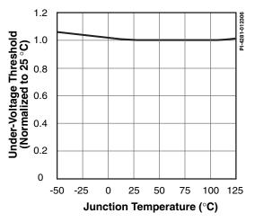
Figure 27. Undervoltage Threshold vs. Temperature.
