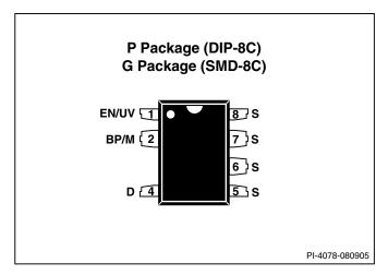
Figure 3. Pin Configuration.
