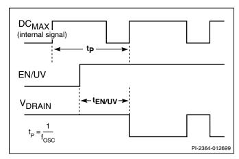
Figure 18. Output Enable Timing.
