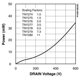
Figure 26. Drain Capacitance Power.
