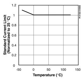
Figure 22. Standard Current Limit vs. Temperature.
