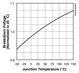
Figure 20. Breakdown vs. Temperature.
