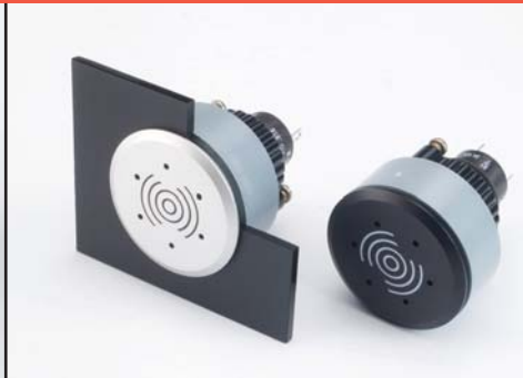
Buzzer, plastic bezel, flush mount, 30.5mm mounting, 24VDC, IP40, 95dB ± 8 at a distance of 0.1m
