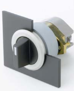
Selector switch, short lever multi position, flush mount, 30.5mm mounting
