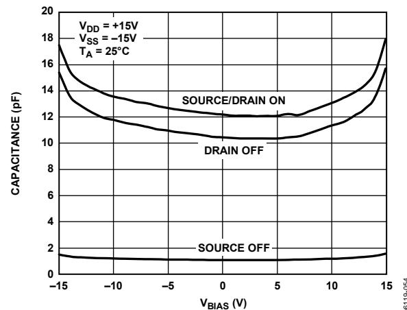
Figure 23. ADG1206 Capacitance vs. Source Voltage,  $\pm 15\text{V}$  Dual Supply
