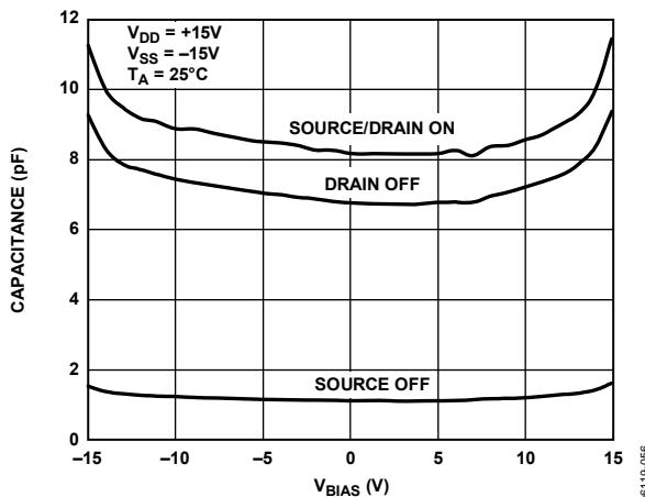
Figure 25. ADG1207 Capacitance vs. Source Voltage,  $\pm 15$  V Dual Supply
