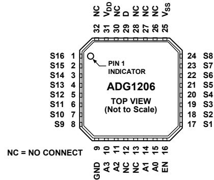
Figure 4. ADG1206 Pin Configuration—5 mm × 5 mm LFCSP\_VQ, Exposed Pad Tied to Substrate,  $V_{SS}$
