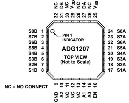
Figure 6. ADG1207 Pin Configuration—5 mm x 5 mm LFCSP\_VQ Exposed Pad Tied to Substrate,  $V_{SS}$
