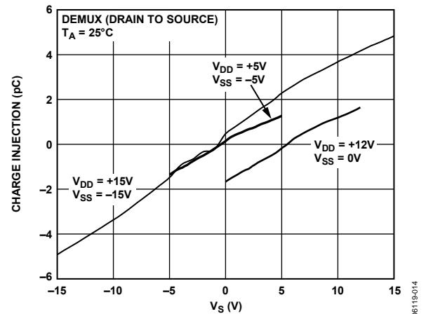
Figure 16. Drain-to-Source Charge Injection vs. Source Voltage
