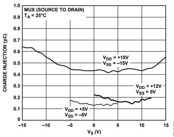
Figure 15. Source-to-Drain Charge Injection vs. Source Voltage
