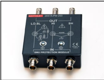
2657A-PM-200: 200V protection module to protect standard triax instruments from 2657A, standard and HV triax cables (3kV rated).
