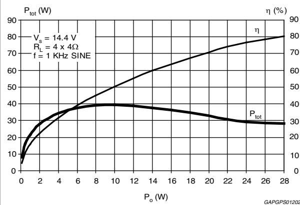
**Figure 15. Power dissipation and efficiency vs. output power ( $R_L = 2 \Omega$ , SINE)**
