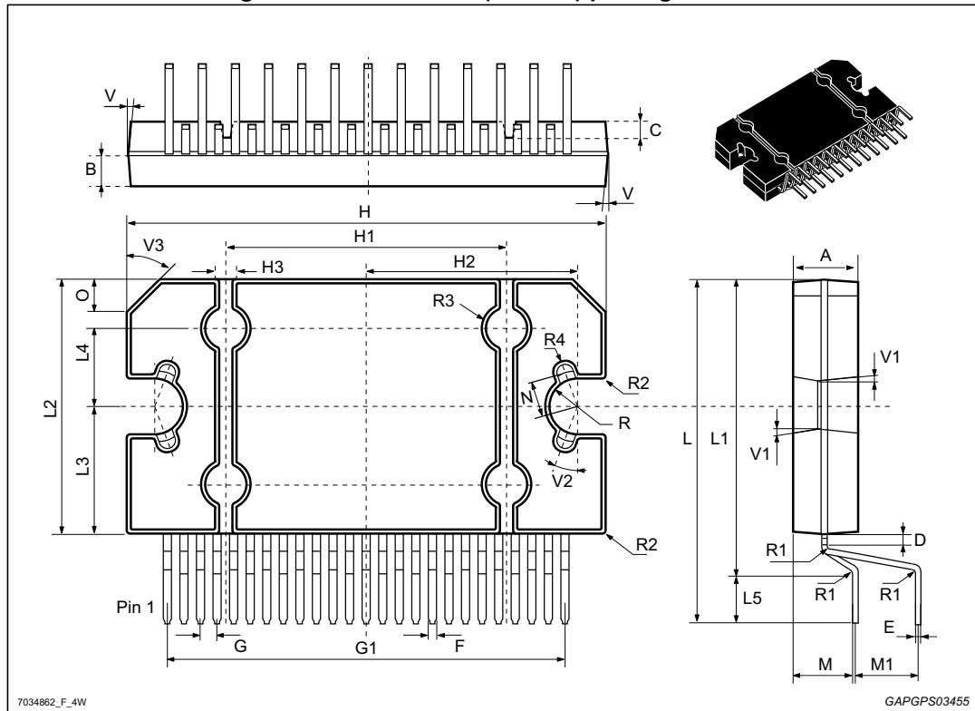
Table 5. Flexiwatt 25 (vertical) package mechanical data
