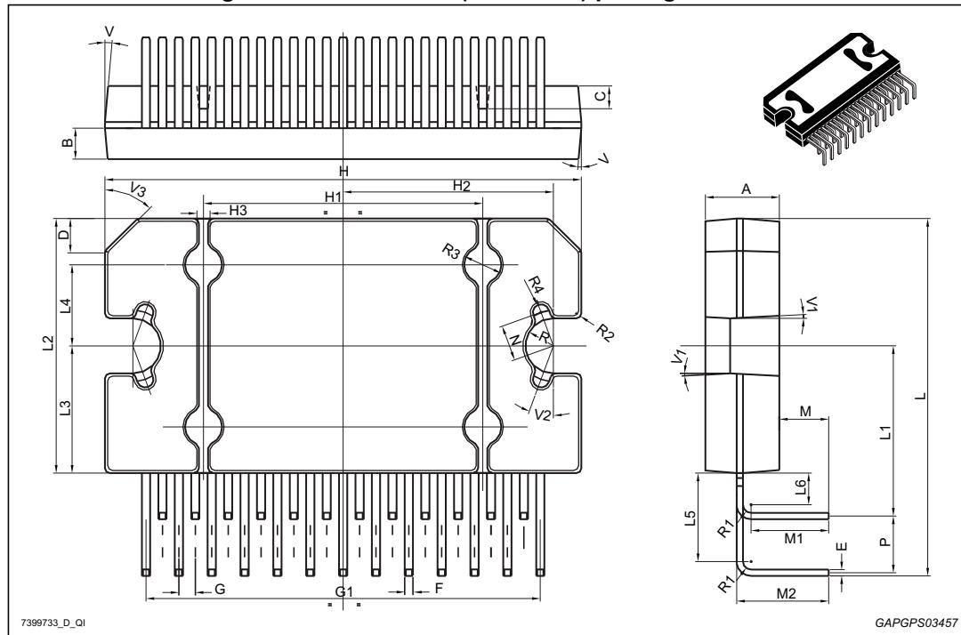
Table 6. Flexiwatt 25 (horizontal) package mechanical data
