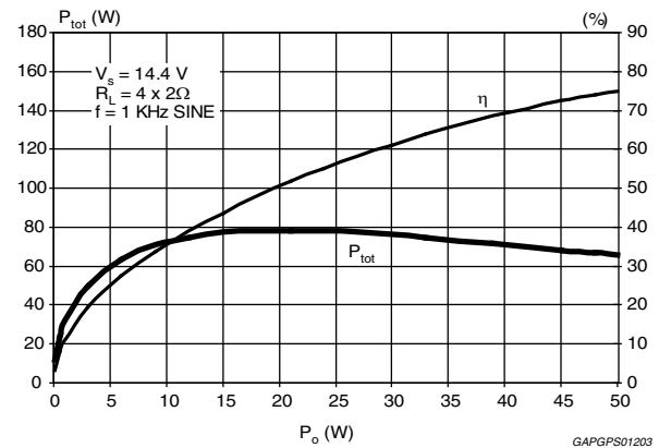
**Figure 16. Power dissipation vs. output power ( $R_L = 4 \Omega$ , audio program simulation)**
