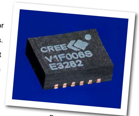
Package Type: 3x4 DFN PN: CGHV1F006S
