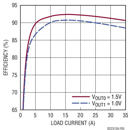
Figure 5. DC2312A-A, Typical Efficiency Curves,
