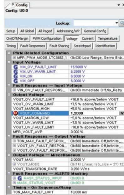
Then, click the "W" (PC to RAM) icon to write these register values to the LTC3882-1. After finishing this step, you will see the output voltage will change to 1.2V.
