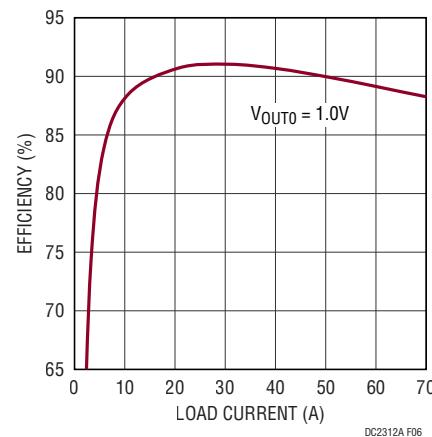
Figure 6. DC2312A-B, Typical Efficiency Curves,
