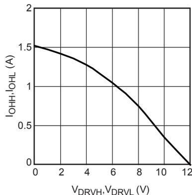
**Peak Pull-down Current vs. Output Voltage**
