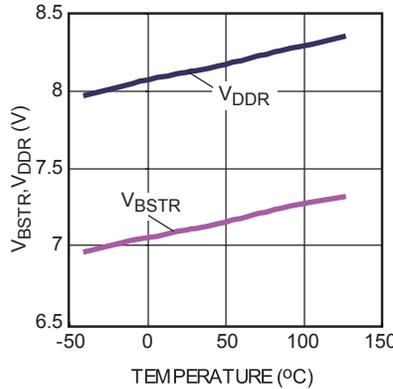
**Undervoltage Lockout Hysteresis vs. Temperature**
