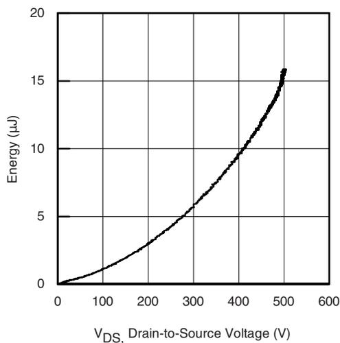
Fig. 6 - Typ. Output Capacitance Stored Energy vs.  $V_{DS}$
