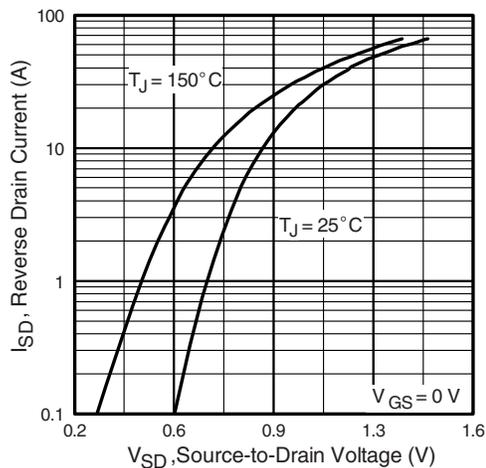
Fig. 8 - Typical Source-Drain Diode Forward Voltage
