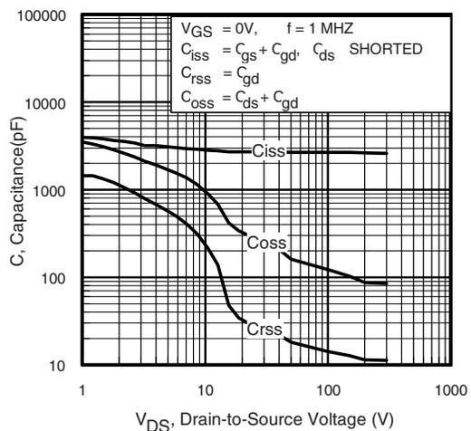
Fig. 5 - Typical Capacitance vs. Drain-to-Source Voltage
