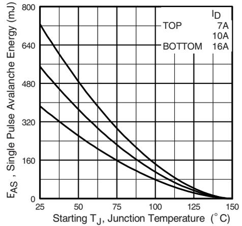
Fig. 13 - Maximum Avalanche Energy vs. Drain Current
