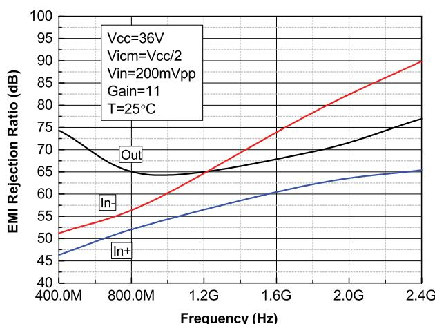
EMIRR performance might be improved by adding small capacitances (in the pF range) on the inputs, power supply and output pins. These capacitances help in minimizing the impedance of these nodes at high frequencies.
