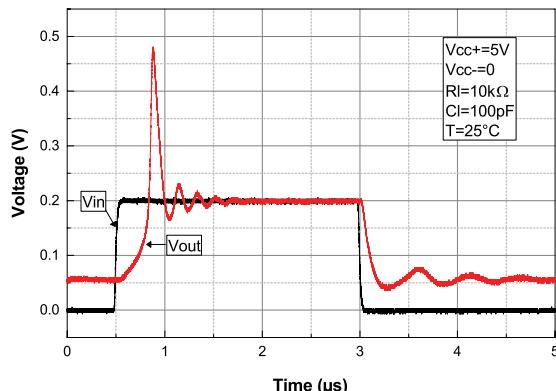
**Figure 30. Desaturation time at high rail at  $V_{CC} = 5$  V**
