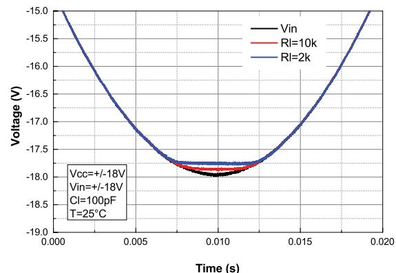
**Figure 33. Amplifier behavior close to the high rail at  $V_{CC} = 36$  V**
