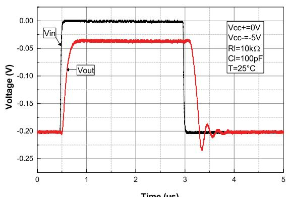
**Figure 31. Small step response vs. time at  $V_{CC} = 36$  V**
