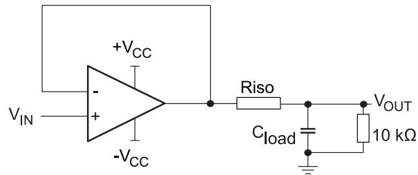
Please note that  $R_{ISO} = 30 \Omega$  is sufficient to make the TSB712A/TSB712 stable whatever the capacitive load.
