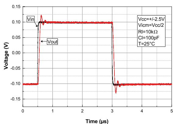
**Figure 29. Desaturation time at low rail at  $V_{CC} = 5$  V**
