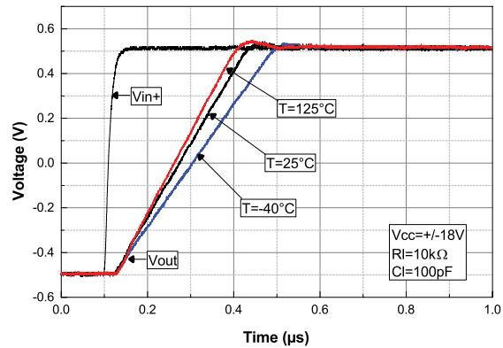
**Figure 21. Negative slew rate at  $V_{CC} = 36 \text{ V}$**
