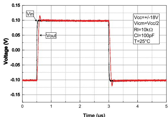
**Figure 32. Amplifier behavior close to the low rail at  $V_{CC} = 36$  V**
