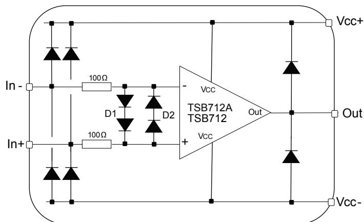
When the input pin voltage exceeds the power supply, the ESD diodes become conductive and, depending on this voltage, excessive current can flow through them. Without limitation this overcurrent can damage the device. In this case, the current has to be limited to 10 mA by adding a resistance in series with the input pin.
