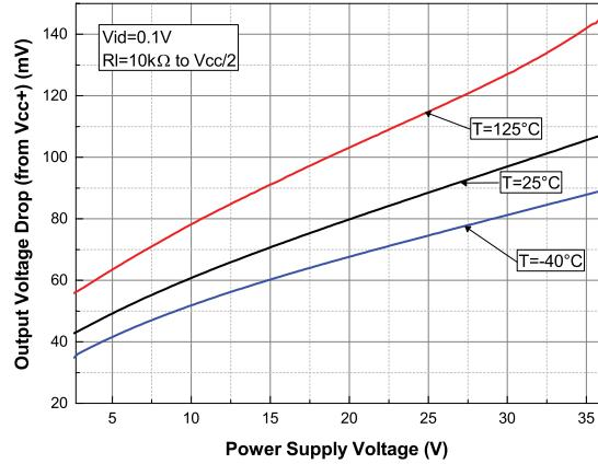
**Figure 19. Output voltage ( $V_{OL}$ ) vs. supply voltage**
