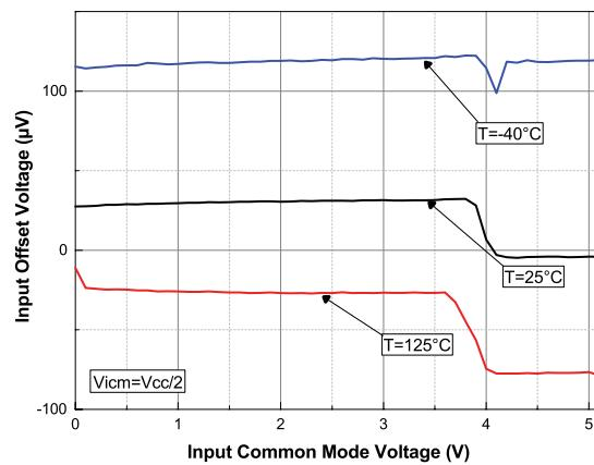
**Figure 12. Input offset voltage vs. common mode voltage at  $V_{CC} = 36$  V TSB712A**
