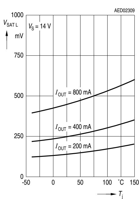
**Total Drop at outputs  $V_{SAT}$  over Temperature**
