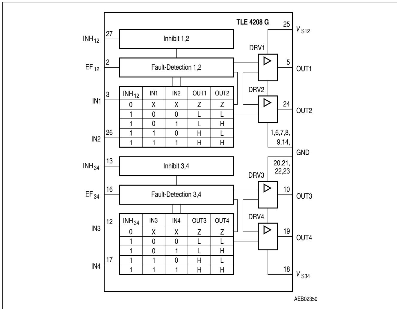
**Figure 1 Block Diagram**
