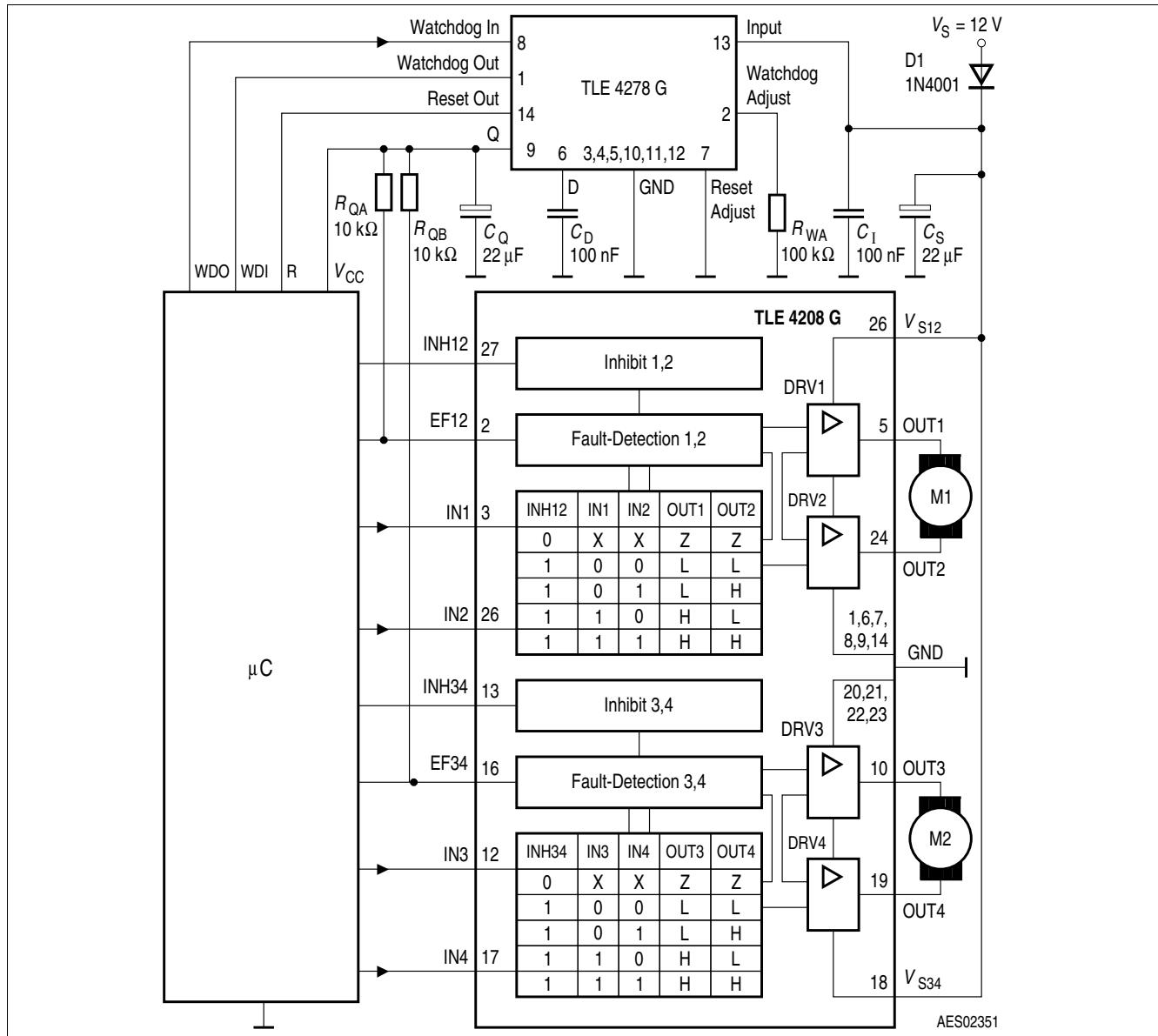
**Figure 3 Application Circuit 1 (Device is used as Dual-Full-Bridge-Driver)**
