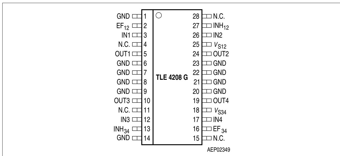
Figure 2 Pin Configuration
