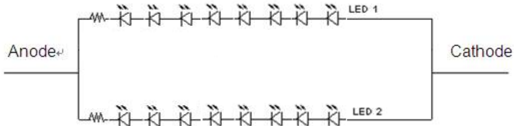
Figure 5 LED Light Bar Structure
