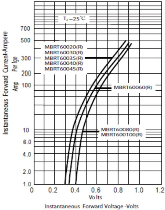
Figure.2-Forward Derating Curve
