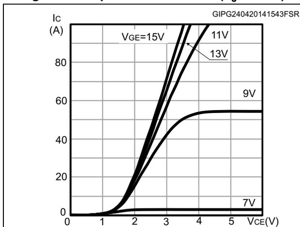
Figure 5. Output characteristics (T<sub>J</sub> = 175°C)
