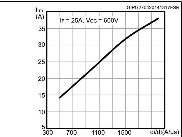
Figure 22. Reverse recovery time vs. diode current slope
