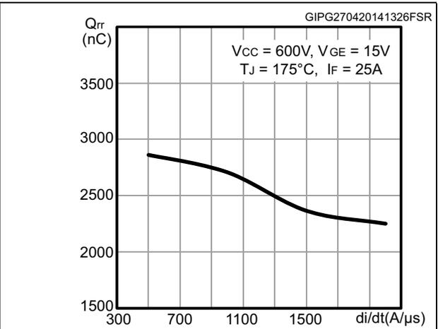
Figure 24. Reverse recovery energy vs. diode current slope
