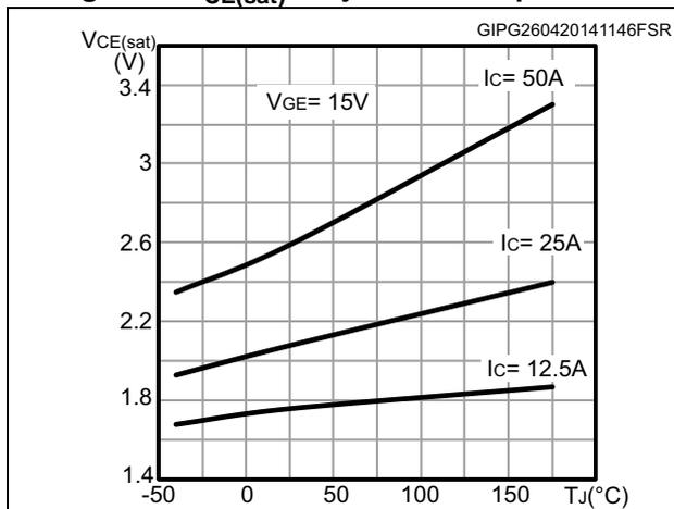
Figure 7. V<sub>CE(sat)</sub> vs. collector current
