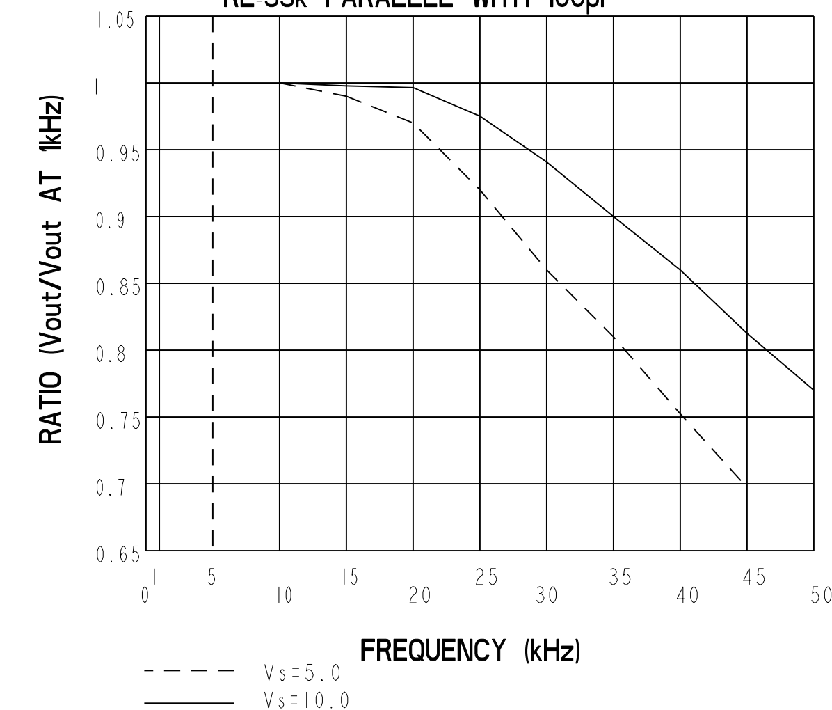
TYPICAL FREQUENCY RESPONSE RL-33k PARALLEL WITH 100pF
