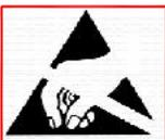
OBSERVE PRECAUTION FOR HANDLING ELECTROSTATIC DISCHARGE SENSITIVE DEVICES
