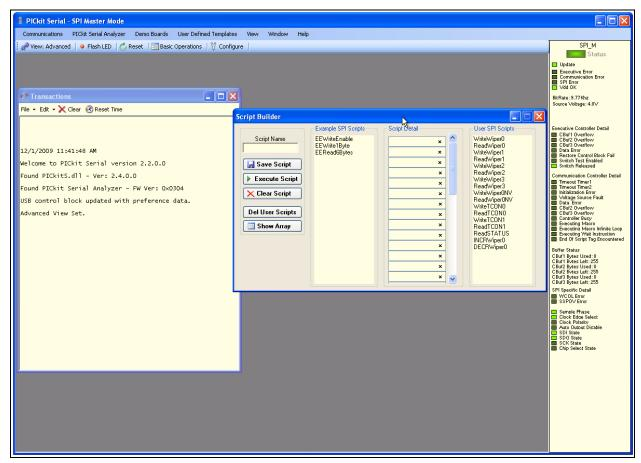
FIGURE 2-9: PICkit™ Serial Main Window at Start-up.
