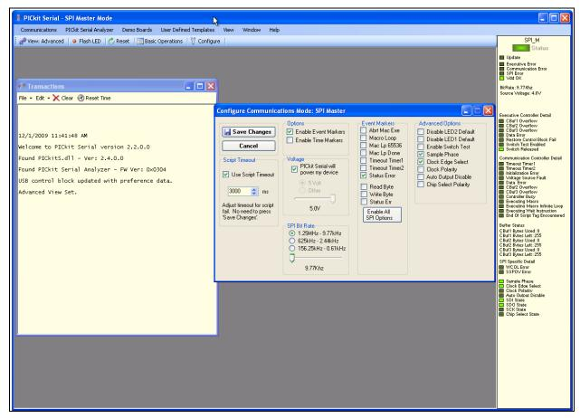
FIGURE 2-7: PICkit™ Serial Configure Communications Mode Window.
