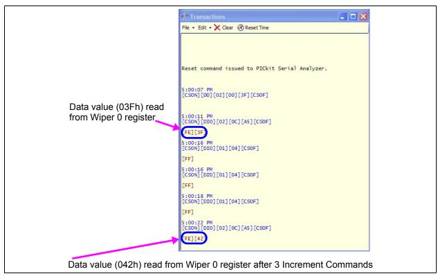
FIGURE 2-15: MCP4261 Transaction Window – Wiper 0 Increments.
