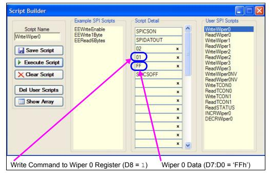
FIGURE 2-12: MCP42XX Write Wiper 0 Script File – Updating Wiper Value.
