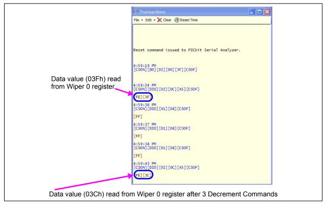
FIGURE 2-14: MCP4261 Transaction Window – Wiper 0 Decrements.
