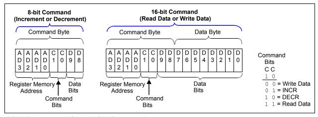
FIGURE 2-3: MCP42XX SPI Command Formats.
