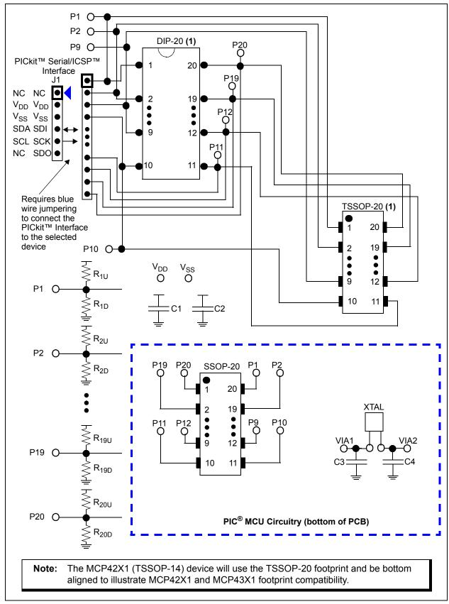
FIGURE 2-1: TSSOP20EV Evaluation Board Circuit.
