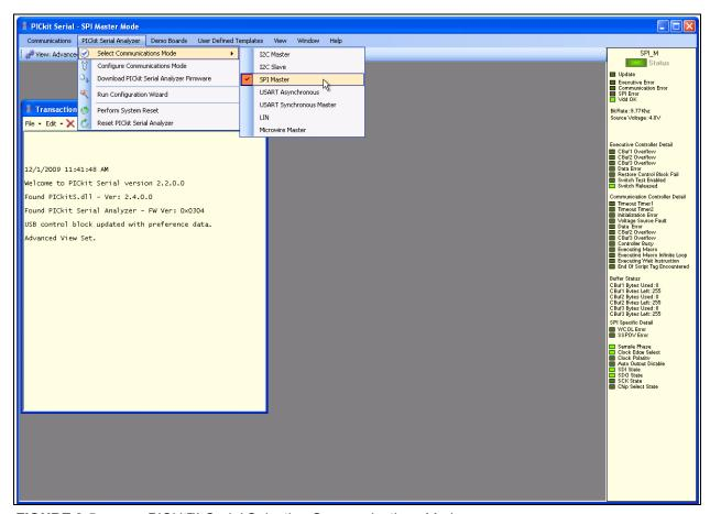
FIGURE 2-5: PICkit™ Serial Selecting Communications Mode.
