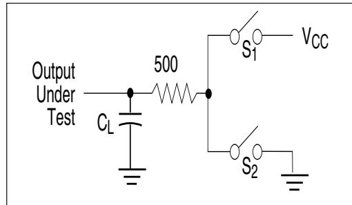
Figure 4. RS-485 Driver Timing Test Load #2 Circuit
