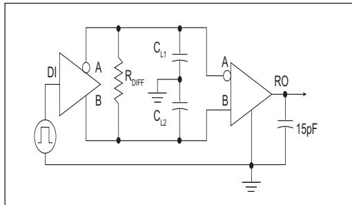
Figure 3. RS-485 Driver/Receiver Timing Test Circuit
