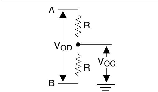
Figure 1. RS-485 Driver DC Test Load Circuit
