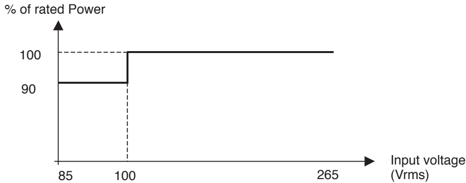
Fig 13-1: Output Power derating at parallel operation
