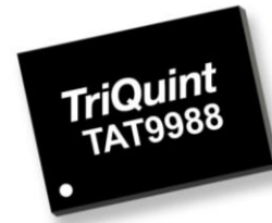
40 Pin 5x7 mm QFN Package
