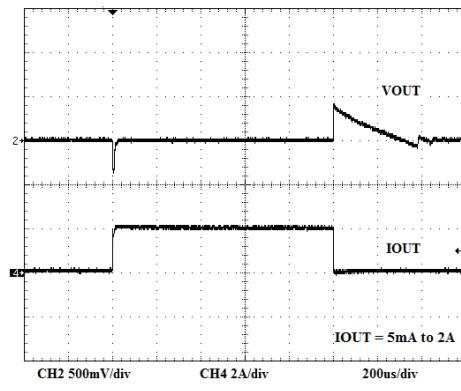
Fig. 13: Load Transient Response at  $V_{OUT}=1.8V$ ,  $V_{IN}=2.8V$
