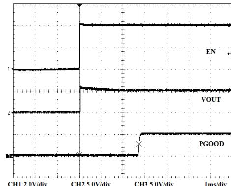
Fig. 18: Enable Startup at  $V_{OUT} = 5V$
