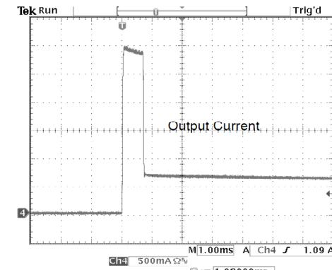
Fig. 21: Current Foldback at  $V_{OUT} = 3.3V$
