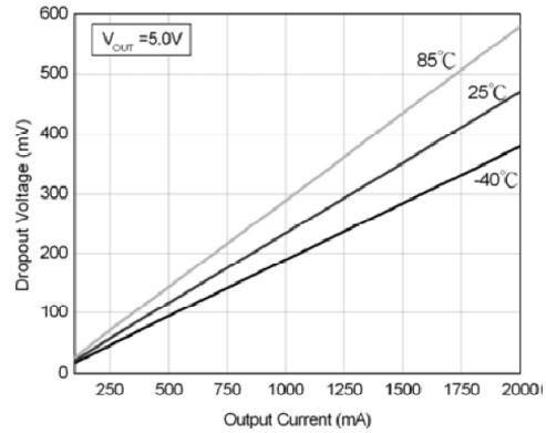
Fig. 12: Dropout Voltage at  $V_{OUT} = 5.0V$
