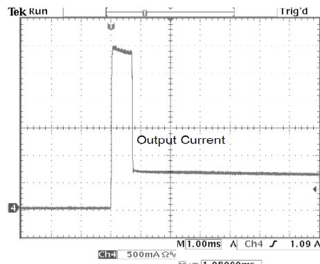
Fig. 20: Current Foldback at  $V_{OUT} = 1.8V$
