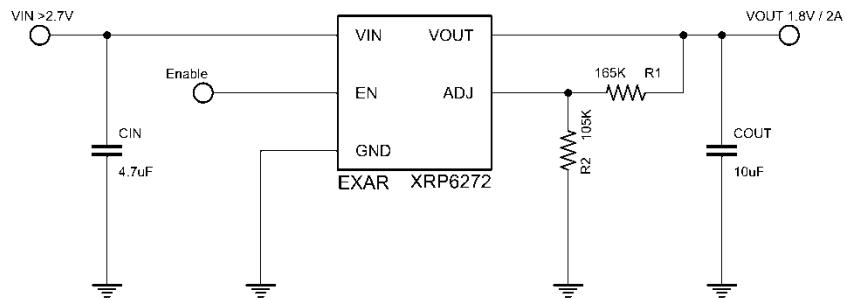
Fig. 25: 2.7V Min to 1.8V / 2A Power Supply
