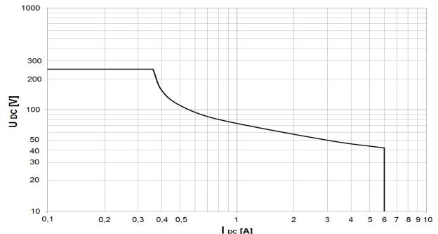
Figure 3 Relay load curve - ohmic load
