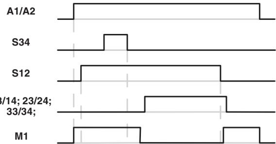
Figure 5 Time diagram for manual, monitored start
