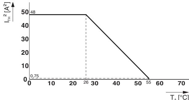
Figure 2 Derating curve - vertical or horizontal mounting position with connected modules
