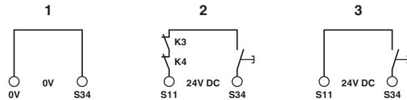
Figure 11 Connection of automatic or manual, monitored start
