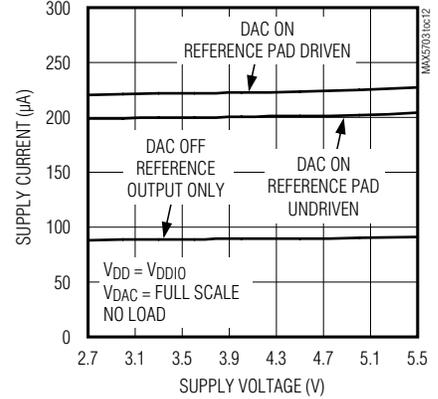
**SUPPLY CURRENT vs. SUPPLY VOLTAGE (2.500V INTERNAL REFERENCE)**
