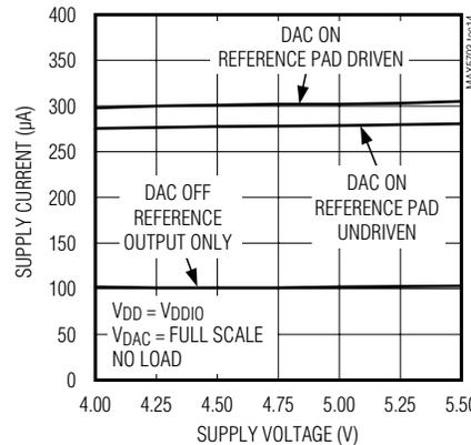
**POWER-DOWN MODE CURRENT vs. SUPPLY VOLTAGE**
