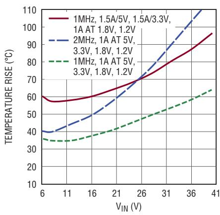
Figure 6. LT8602 Case Temperature Rise,  $T_A = 25^\circ C$
