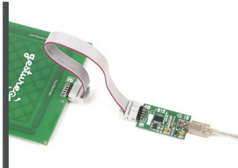
The Gesture board comes with an IDC10 connector cable. If you wish to use it for hardware prototyping, we suggest you pair it with adapter click. The other options is to develop PC applications. For that purpose we developed the Gesture USB adapter.
