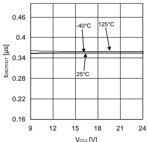
Figure 68. Short Current Detection Delay time (OUT1)
