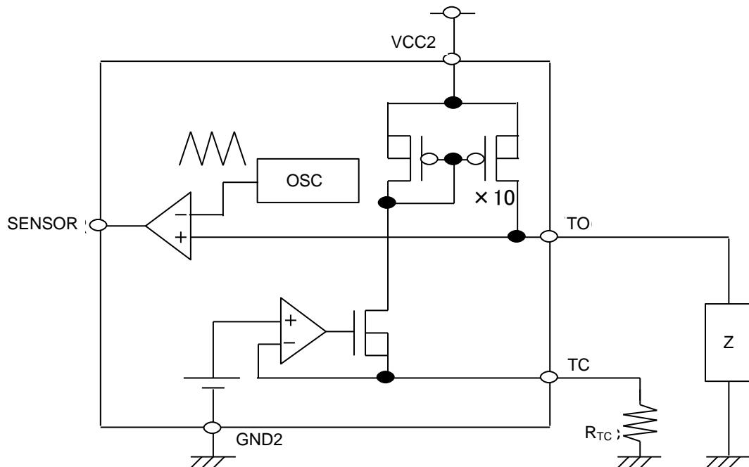
Figure 86. Block Diagram of Temperature Monitor Function
