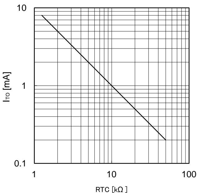
Figure 49. TOx Pin Output Current
