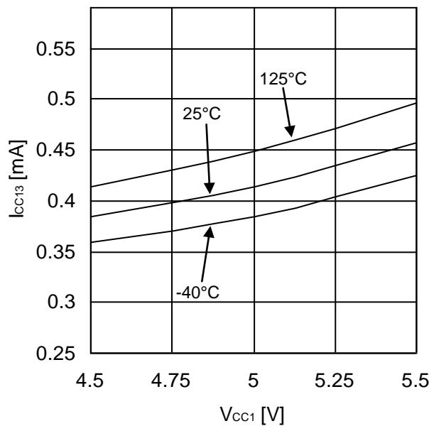
Figure 11. Input Side Circuit Current 3
