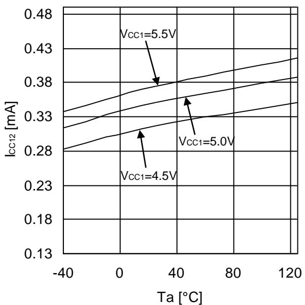
Figure 10. Input Side Circuit Current 2
