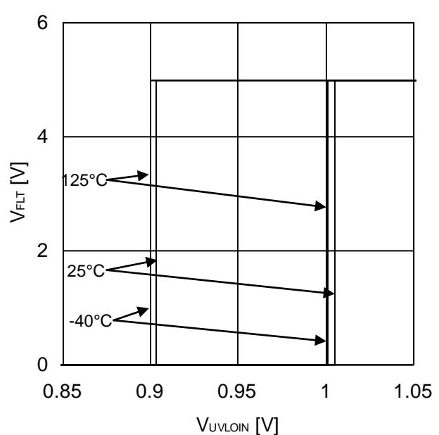
Figure 62. Output-side UVLO ON / OFF Threshold Voltage
