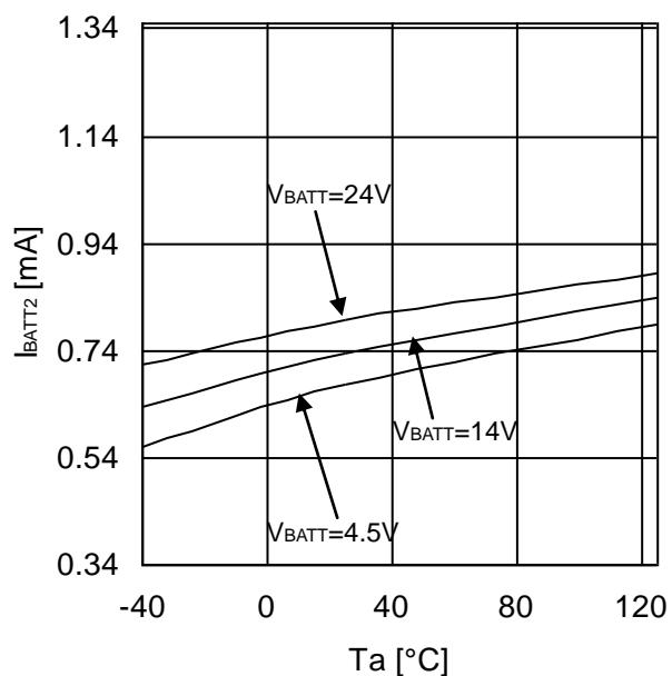
Figure 6. Main Power Supply Circuit Current 2
