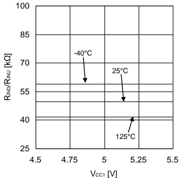
Figure 32. Logic Pull-Down Resistance (INA) Pull-Up Resistance (DIS)
