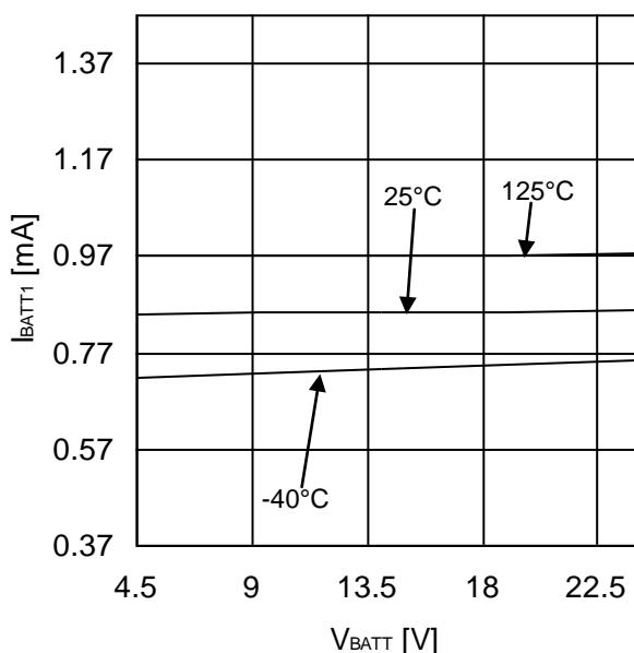
Figure 3. Main Power Supply Circuit Current 1
