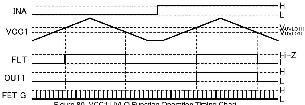
Figure 80. VCC1 UVLO Function Operation Timing Chart
