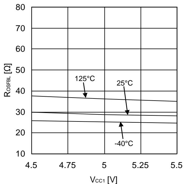
Figure 76. OSFB Output ON-Resistance
