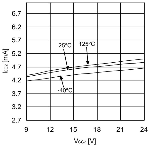
Figure 15. Output Side Circuit Current
