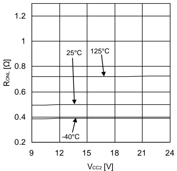
Figure 38. OUT1 ON-Resistance (Sink-side)
