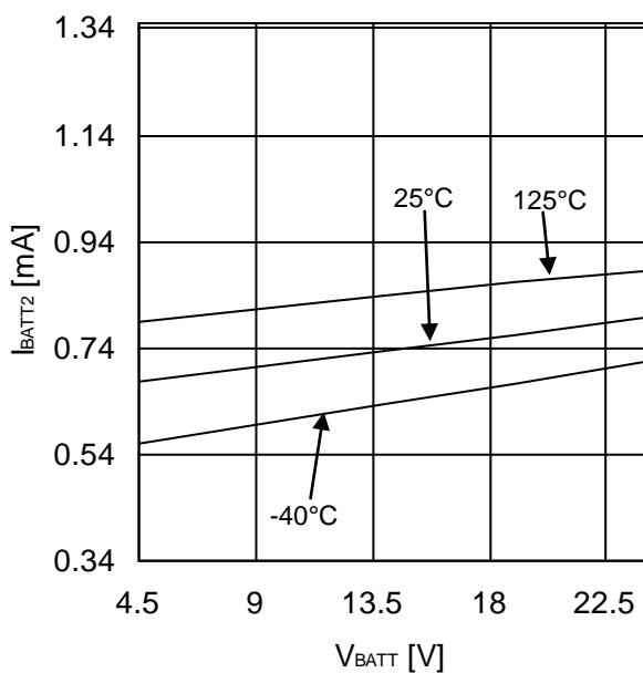
Figure 5. Main Power Supply Circuit Current 2
