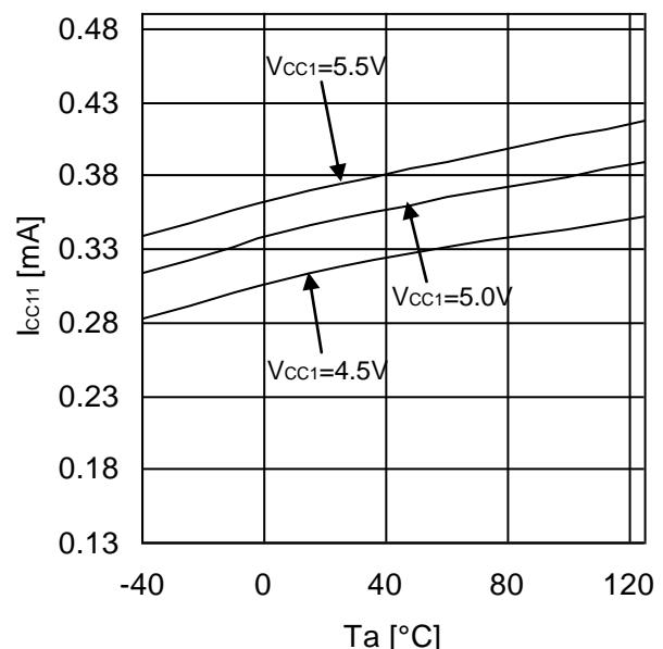
Figure 8. Input Side Circuit Current 1
