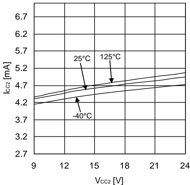
Figure 17. Output Side Circuit Current
