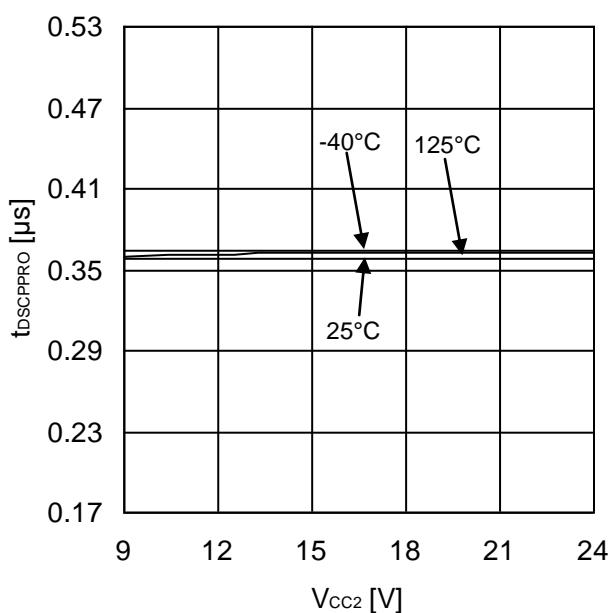
Figure 69. Short Current Detection Delay time (PROOUT)
