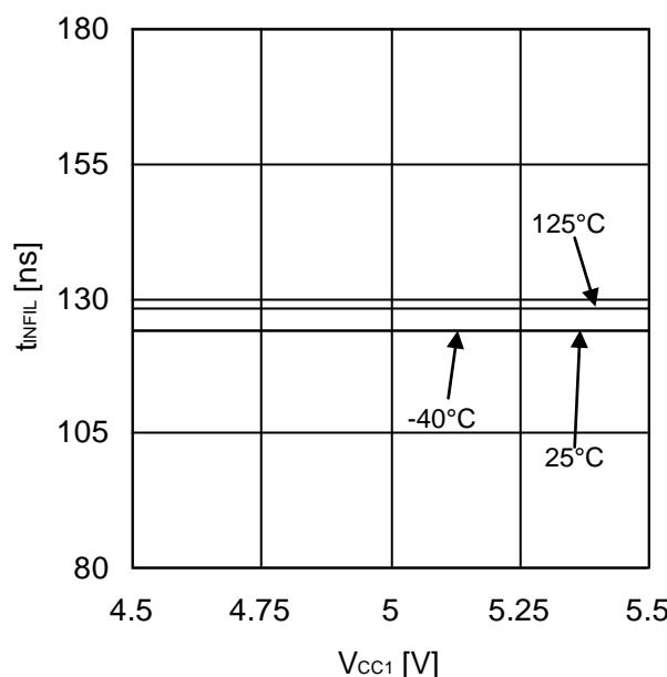
Figure 33. Logic Input Filtering Time (L pulse)
