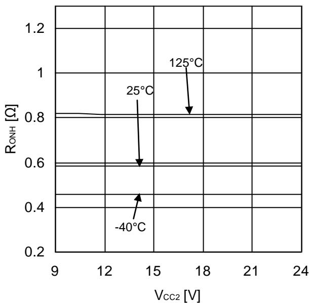
Figure 37. OUT1 ON-Resistance(Source-side)
