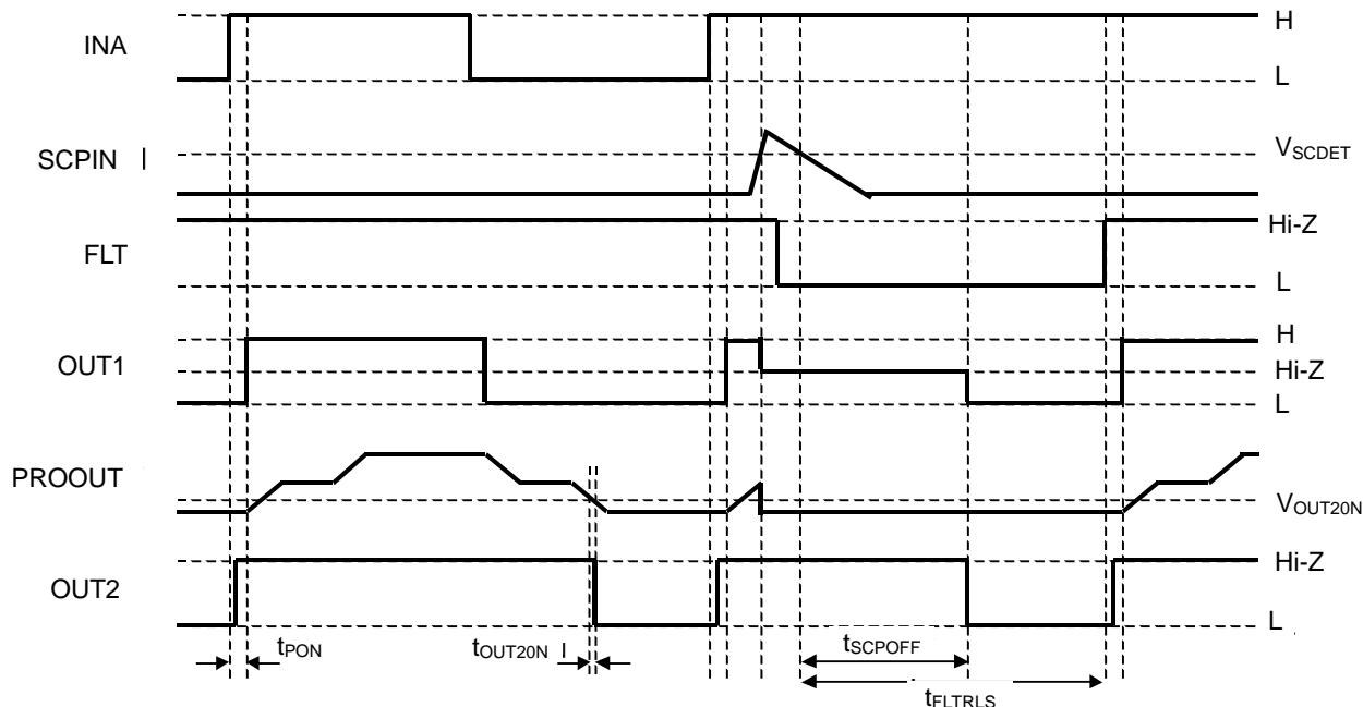
Figure 85. Timing chart of Miller Clamp Function
