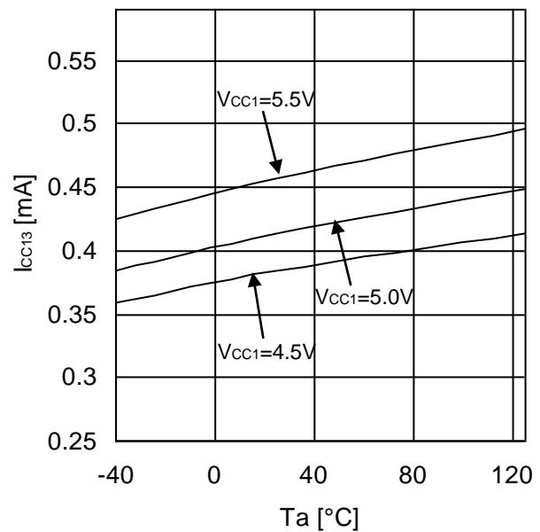
Figure 12. Input Side Circuit Current 3
