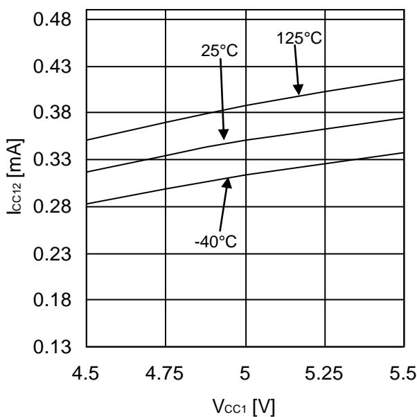
Figure 9. Input Side Circuit Current 2
