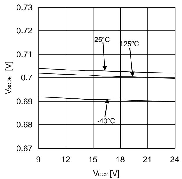
Figure 66. Short Current Detection Voltage
