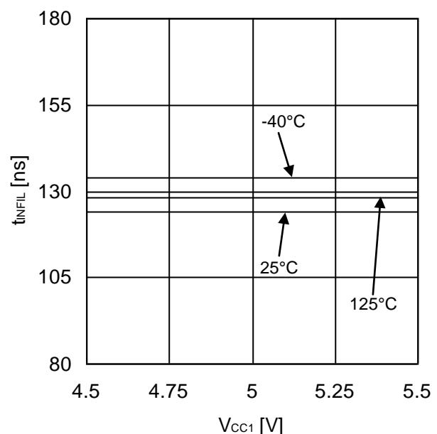
Figure 34. Logic Input Filtering Time (H pulse)
