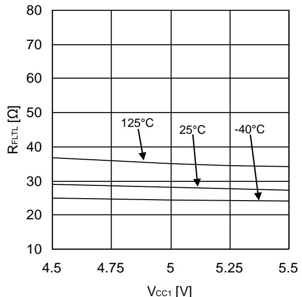
Figure 72. FLT Output ON-Resistance
