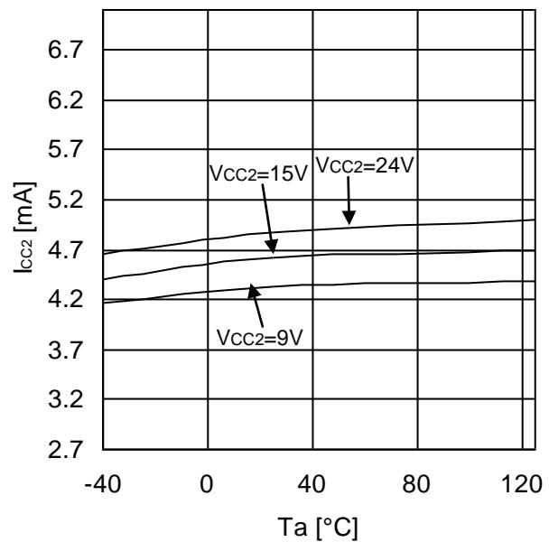
Figure 16. Output Side Circuit Current
