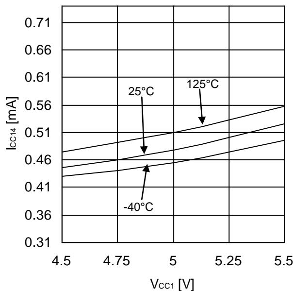
Figure 13. Input Side Circuit Current 4
