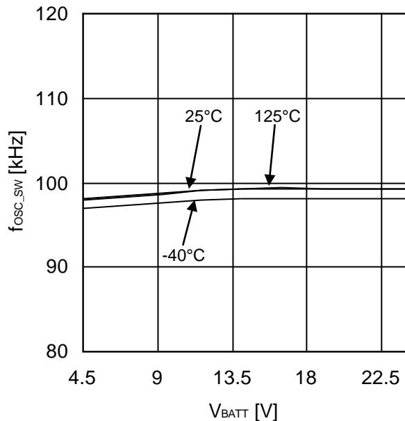
Figure 23. Oscillation Frequency
