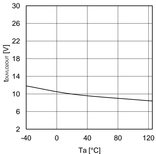
Figure 64. Output-side UVLO Delay Time (OUT1)
