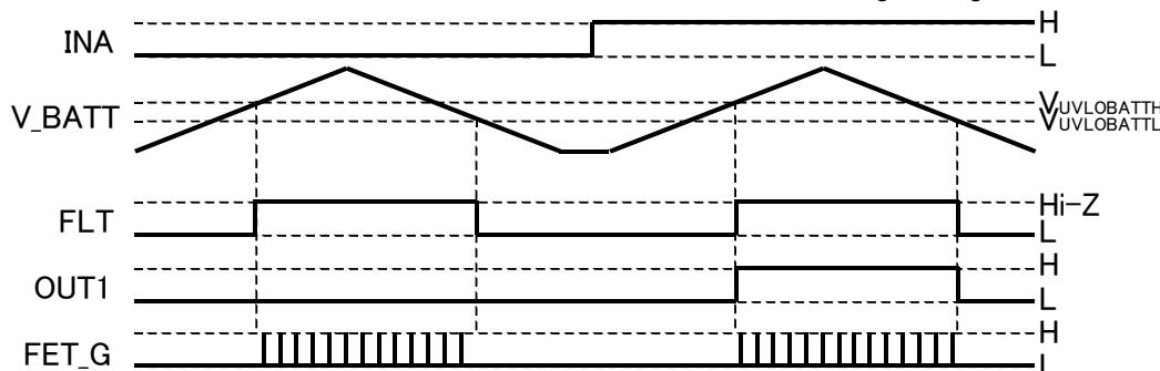
Figure 79. V\_BATT UVLO Function Operation Timing Chart
