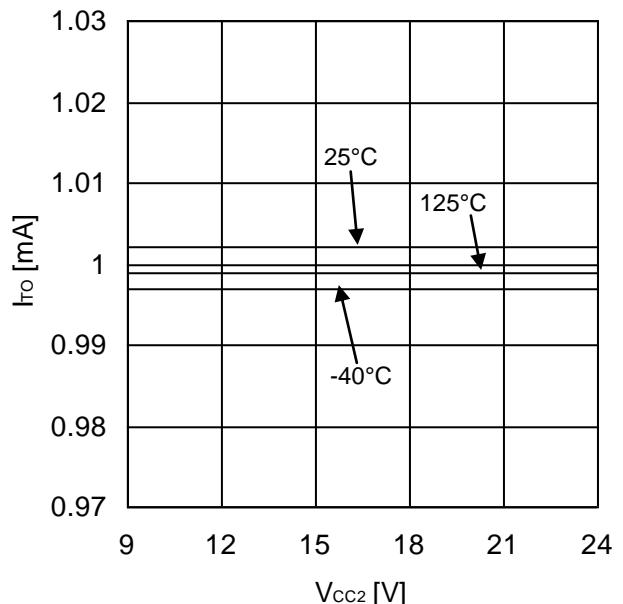
Figure 48. TOx Pin Output Current (RTC=10kΩ)
