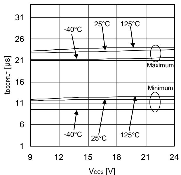
Figure 70. Short Current Detection Delay time (FLT)
