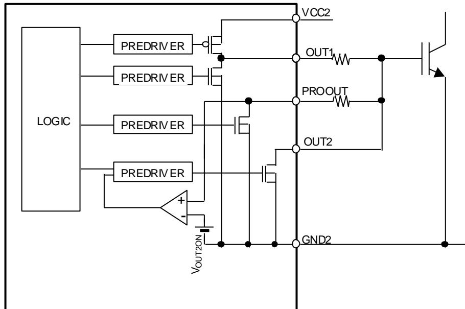
Figure 84. Block Diagram of Miller Clamp Function
