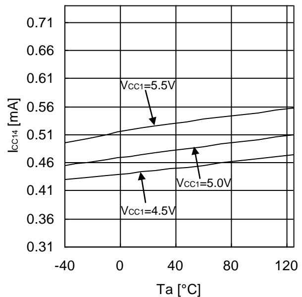
Figure 14. Input Side Circuit Current 4
