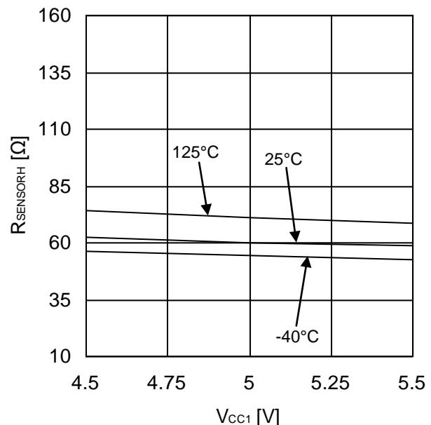
Figure 56. SENSOR ON Resistance(Source-side)
