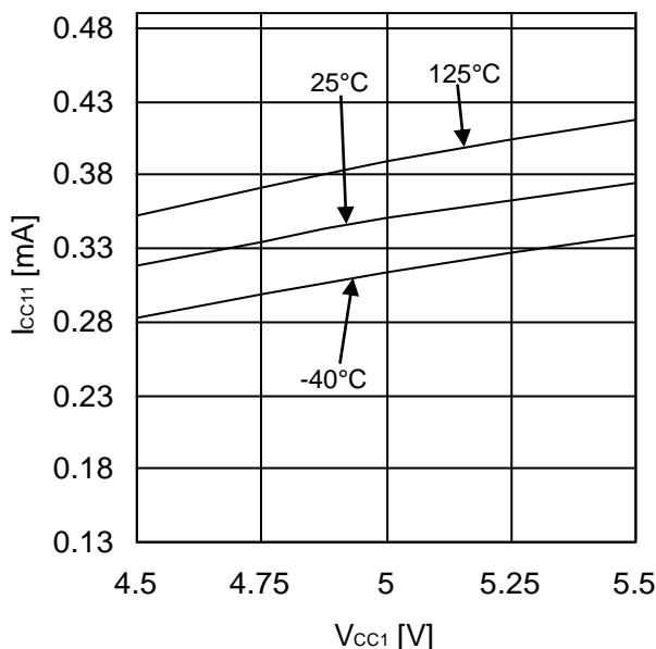
Figure 7. Input Side Circuit Current 1
