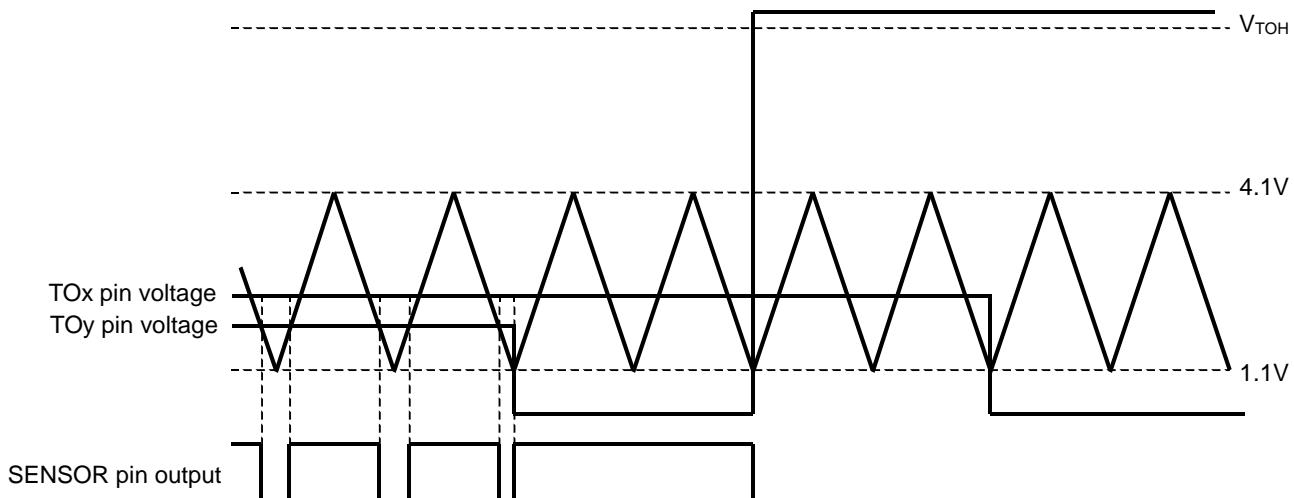
Figure 87. Timing Chart of Temperature Monitor Function
