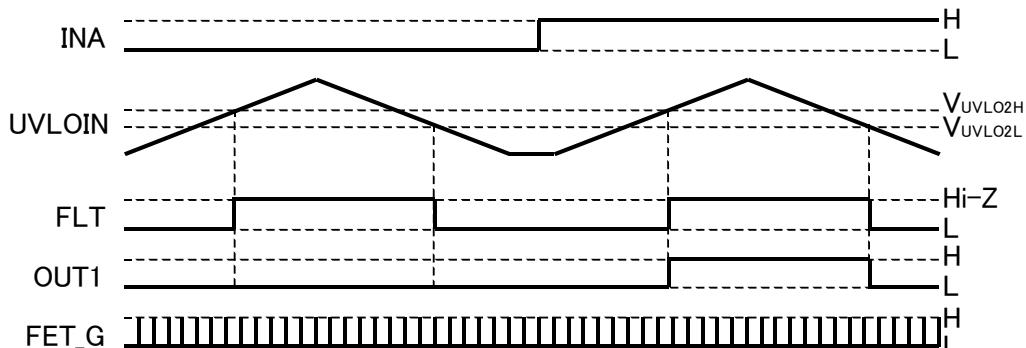
Figure 81. VCC2 UVLO Function Operation Timing Chart
