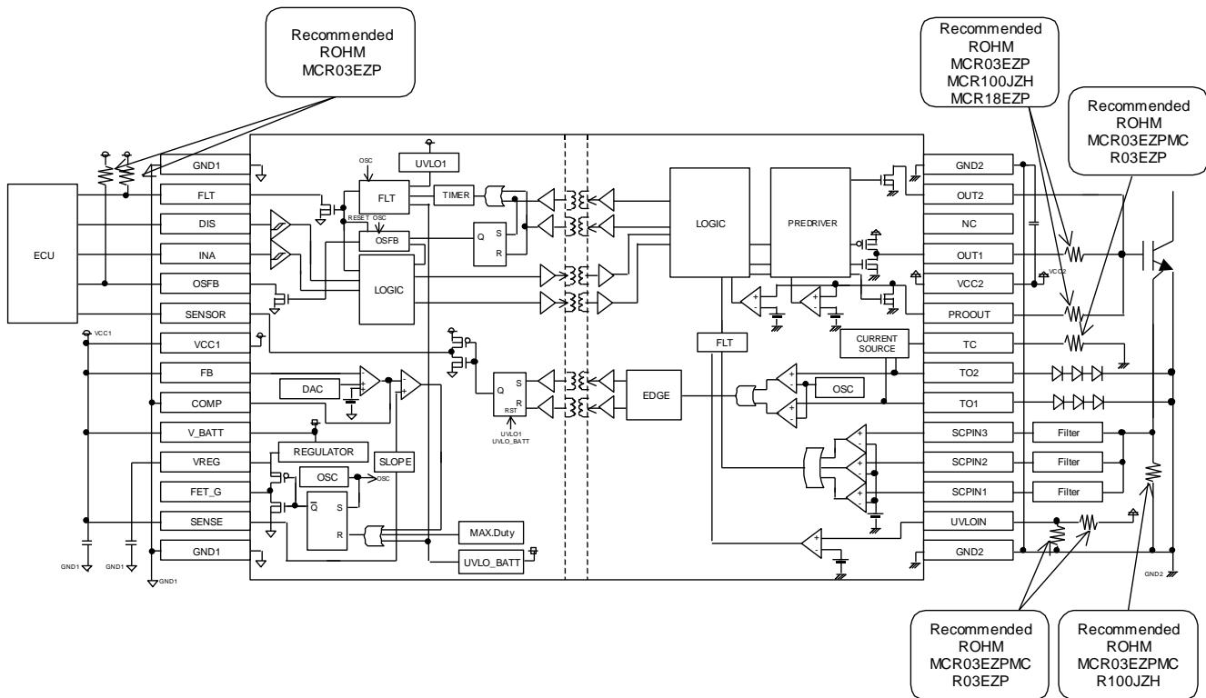
Figure 90. For no using switching power supply controller
