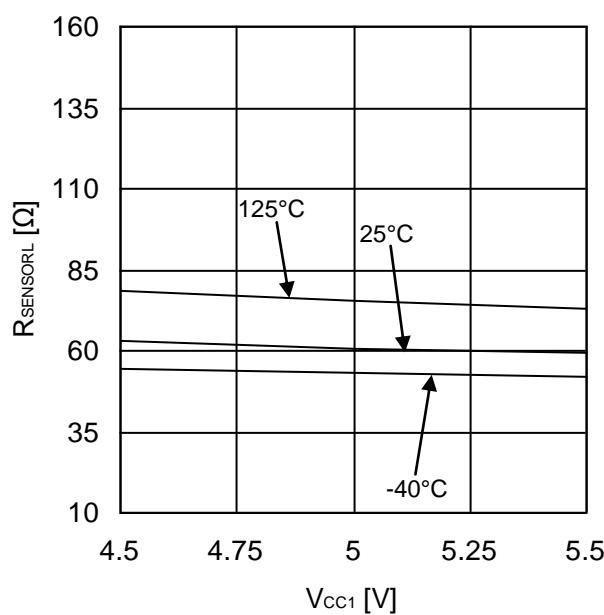
Figure 57. SENSOR ON Resistance (Sink-side)
