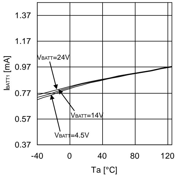
Figure 4. Main Power Supply Circuit Current 1
