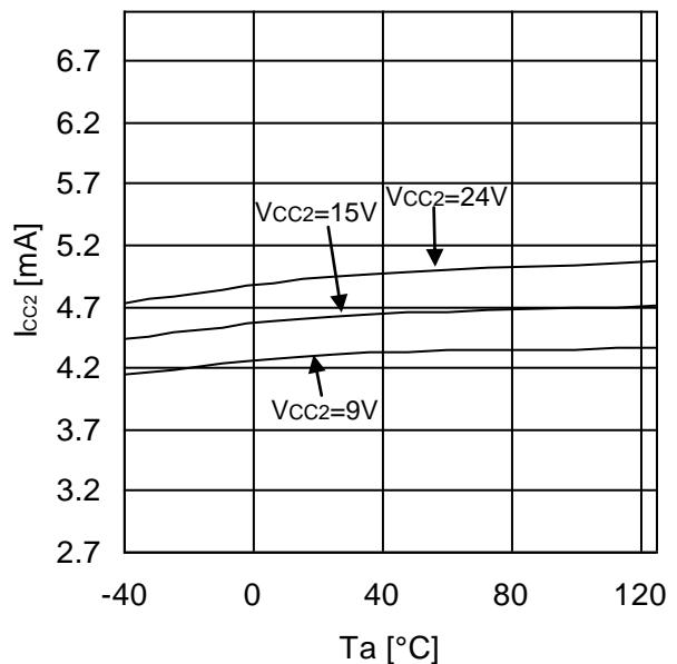
Figure 18. Output Side Circuit Current
