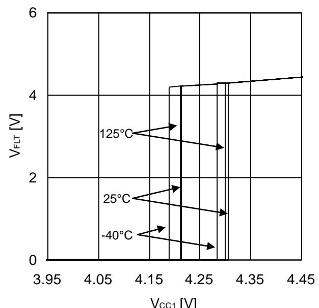
Figure 58. Input-side UVLO ON/OFF Voltage
