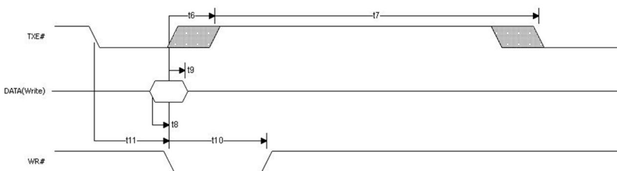
Figure 3.4 – Asynchronous FIFO Mode Read and Write Cycle.
