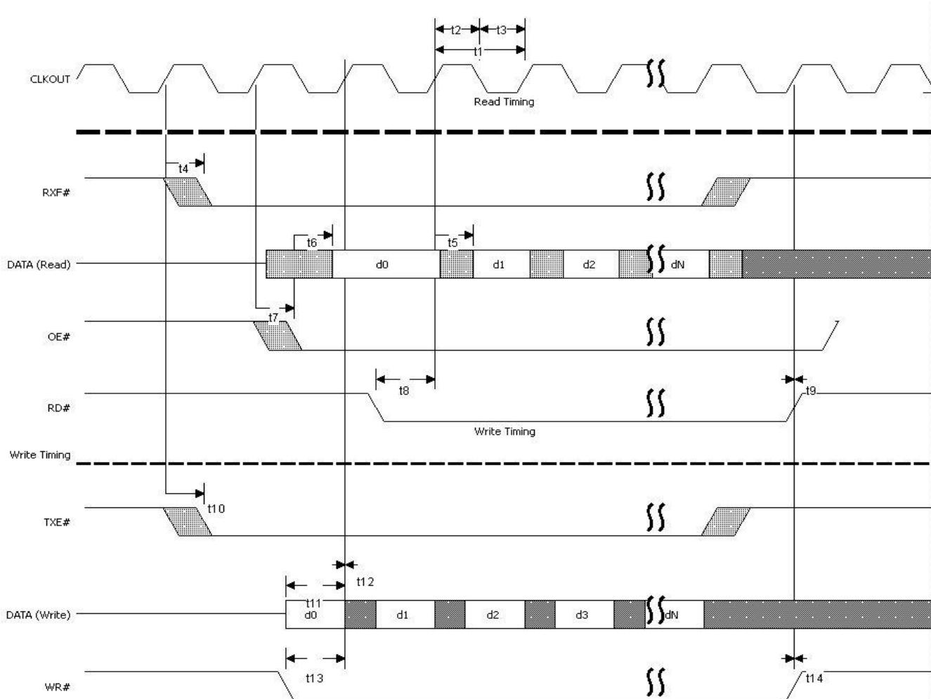
**Figure 3.5 - Synchronous FIFO Mode Read and Write Cycle**
