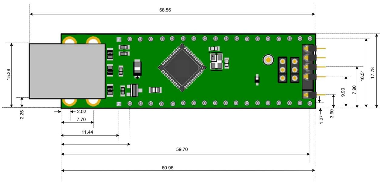
**Figure 5.1 V2DIP2 48 Dimensions (Top View)**
