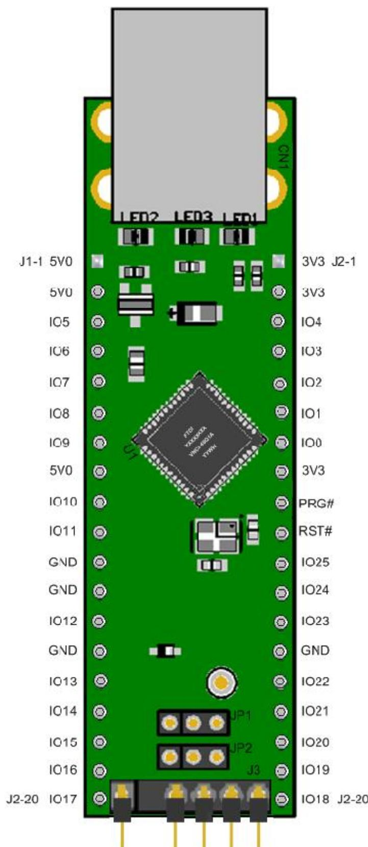
Figure 3.1 - V2DIP2 48 Module Pin Out (Top View)
