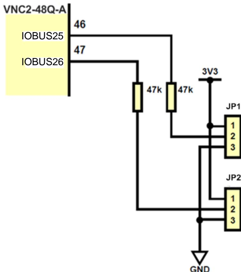
**Figure 3.3 - V2DIP2 48 On-Board Jumper Pin Configuration.**
