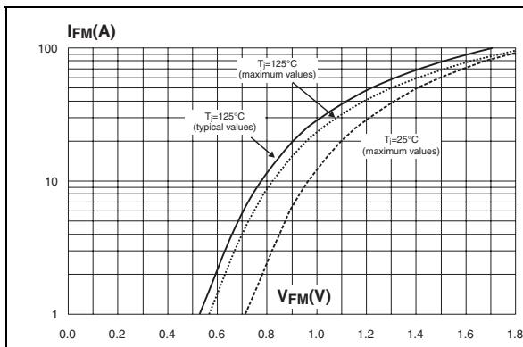
**Figure 10. Forward voltage drop versus forward current**
