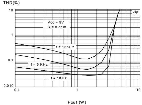
Figure 9. Distortion vs. frequency
