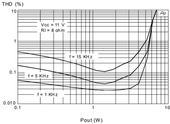
Figure 8. Distortion vs. output power ( $V_{CC} = 9\text{ V}$ )
