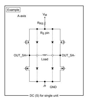
o : Indicates an IC output pin connected to a motor.
