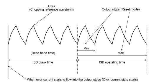
The over-current detection circuit has a dead band time to prevent erroneous detection of  $I_{RR}$  or spike current at switching. The dead band time being synchronized with the frequency of the OSC for setting chopping frequency is expressed as follows.
