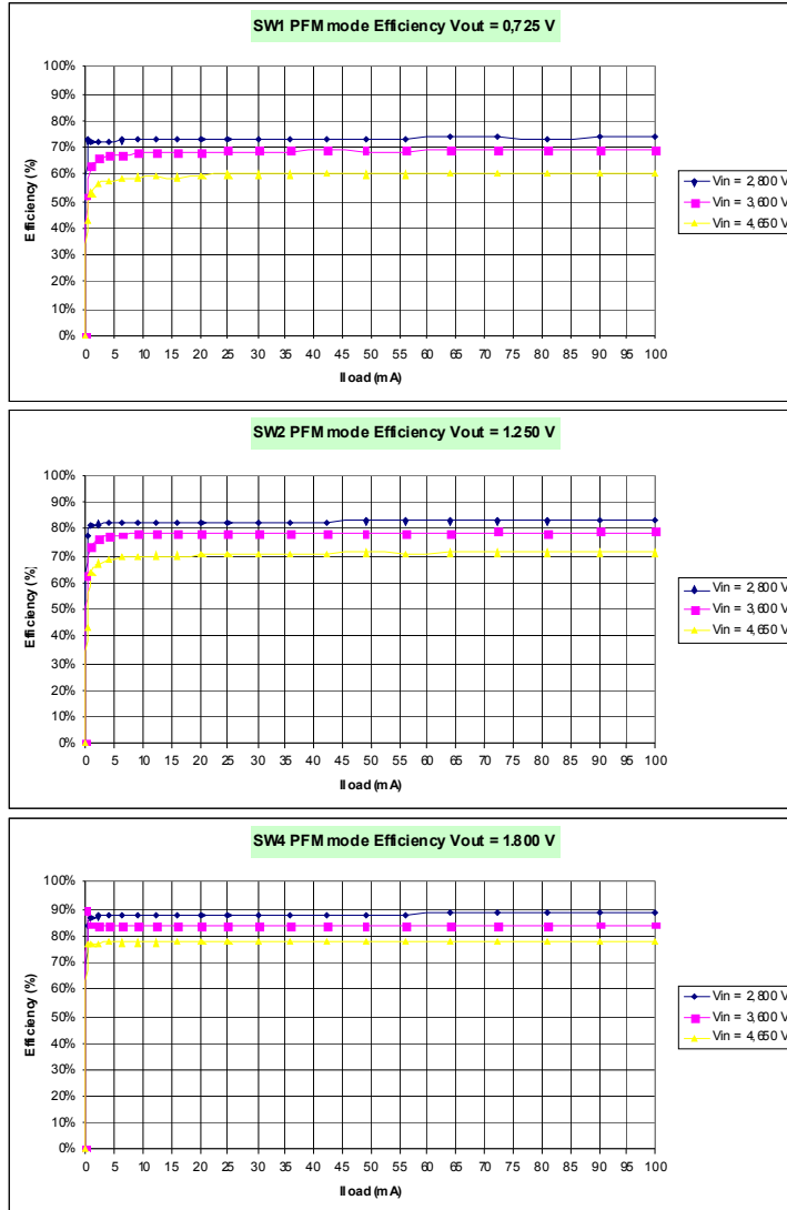
Figure 17. Buck Regulator PFM Efficiency
