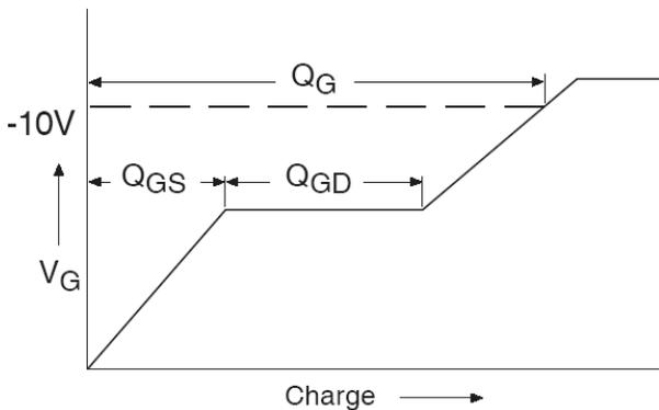
**Fig 13a.** Gate Charge Waveform
