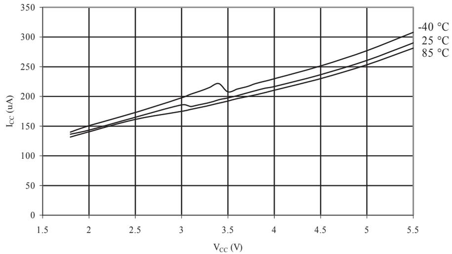
Figure 34-41. ATmega48A: Analog Comparator Current vs. V<sub>CC</sub>
