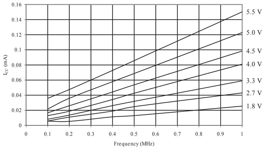
**Figure 34-7. ATmega48A: Idle Supply Current vs. Frequency (1MHz - 20MHz)**
