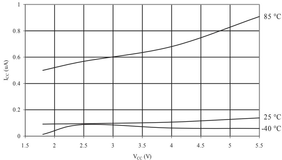
Figure 34-106. ATmega168A: Power-Down Supply Current vs. V<sub>CC</sub> (Watchdog Timer Enabled)
