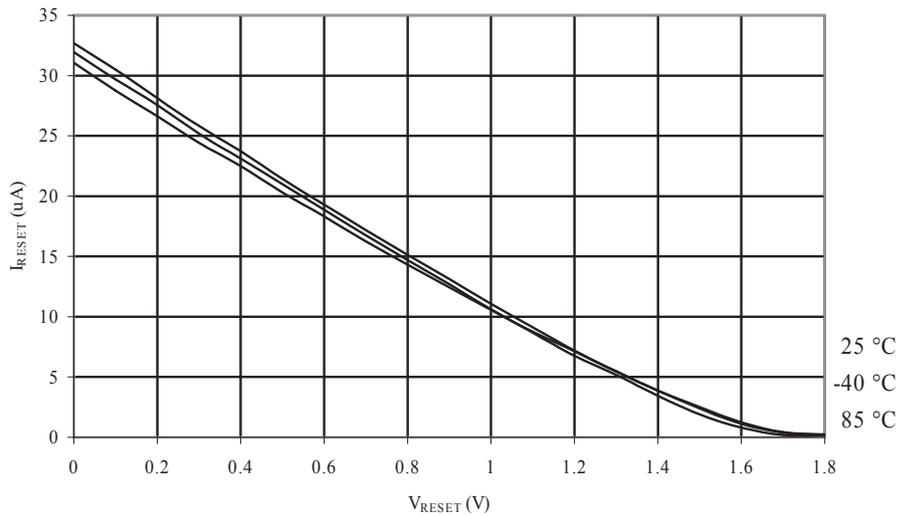
**Figure 34-19. ATmega48A: Reset Pull-up Resistor Current vs. Reset Pin Voltage ( $V_{CC} = 2.7V$ )**
