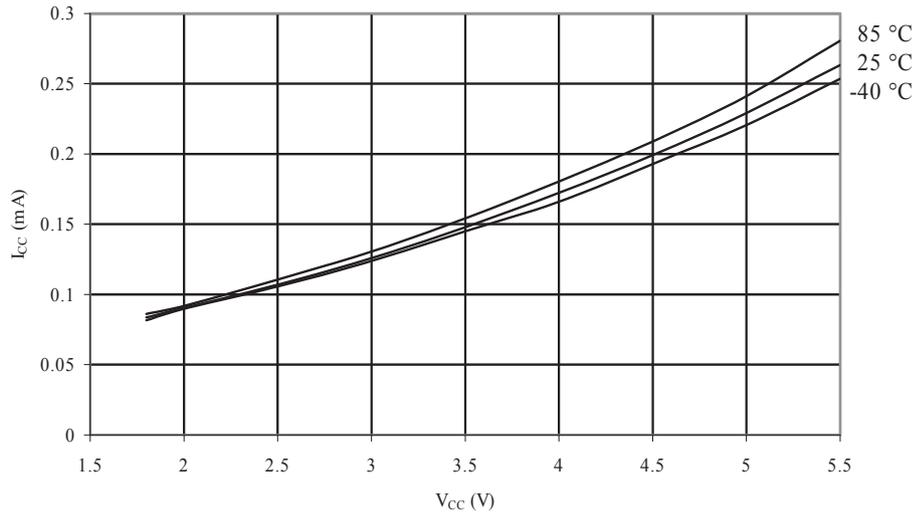
**Figure 34-104. ATmega168A: Idle Supply Current vs.  $V_{CC}$  (Internal RC Oscillator, 8MHz)**
