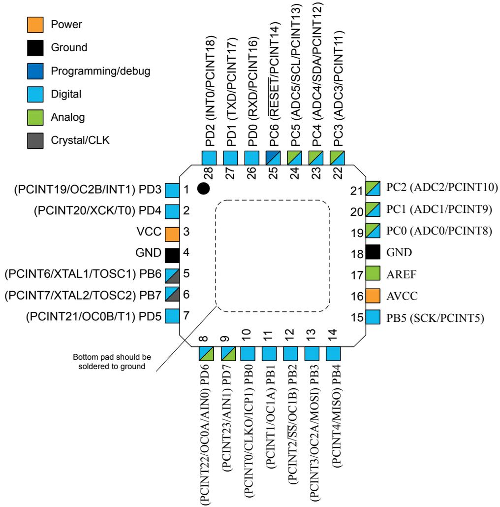
Figure 5-3. 32-pin TQFP Top View
