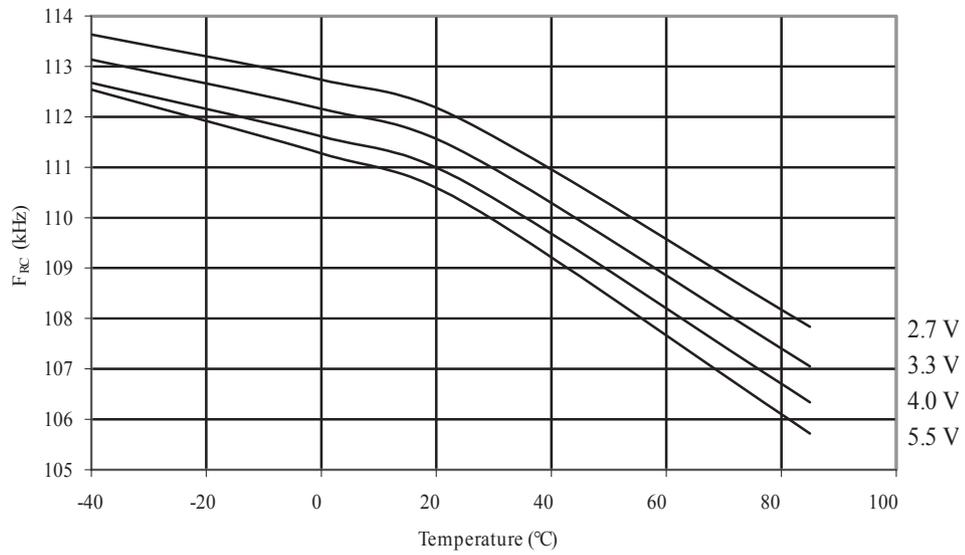
Figure 34-83. ATmega88A: Watchdog Oscillator Frequency vs.  $V_{CC}$
