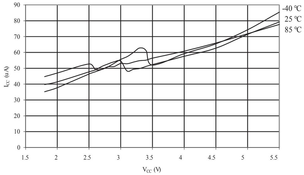
Figure 34-89. ATmega88A: AREF External Reference Current vs.  $V_{CC}$
