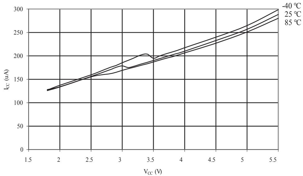
Figure 34-88. ATmega88A: Analog Comparator Current vs.  $V_{CC}$
