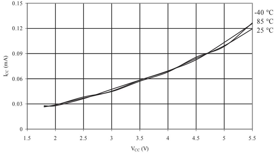
**Figure 34-98. ATmega168A: Active Supply Current vs.  $V_{CC}$  (Internal RC Oscillator, 1MHz)**
