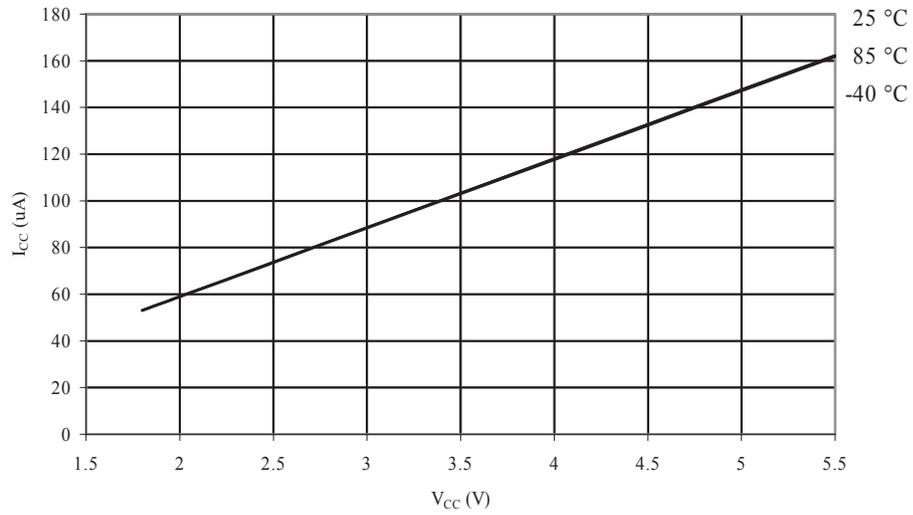
**Figure 34-137. ATmega168A: Brownout Detector Current vs. V<sub>CC</sub>**
