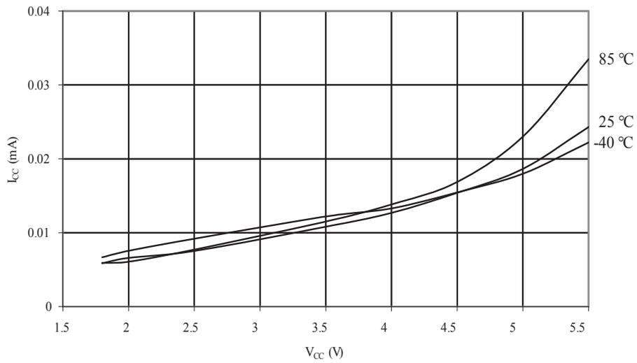
**Figure 34-56. ATmega88A: Idle Supply Current vs. V<sub>CC</sub> (Internal RC Oscillator, 1MHz)**
