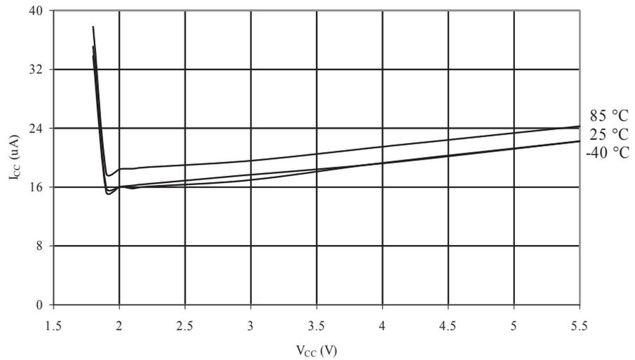
**Figure 34-44. ATmega48A: Programming Current vs. V<sub>CC</sub>**
