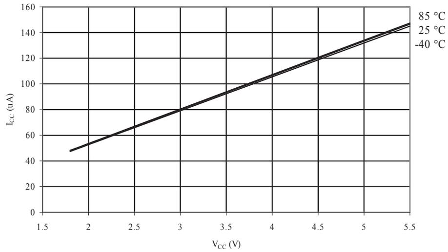
Figure 34-43. ATmega48A: Brownout Detector Current vs. V<sub>CC</sub>
