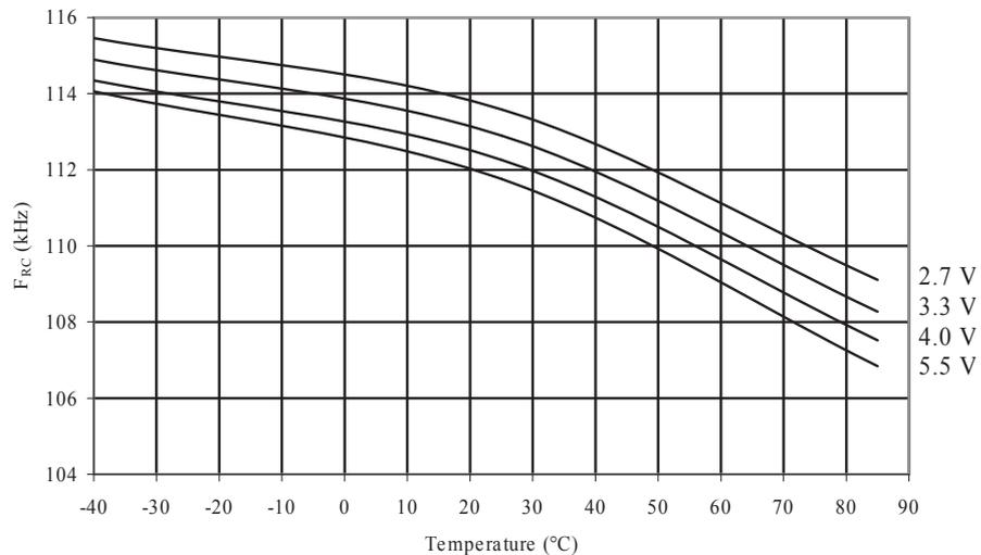
**Figure 34-36. ATmega48A: Watchdog Oscillator Frequency vs.  $V_{CC}$**
