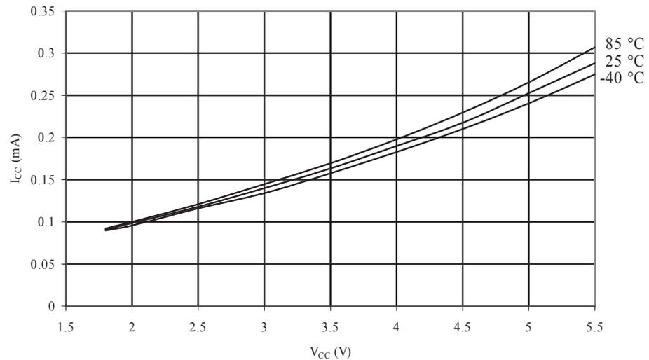
**Figure 34-10. ATmega48A: Idle Supply Current vs. V<sub>CC</sub> (Internal RC Oscillator, 8MHz)**
