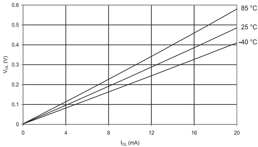
Figure 34-23. ATmega48A: I/O Pin Output Voltage vs. Source Current ( $V_{CC} = 3V$ )
