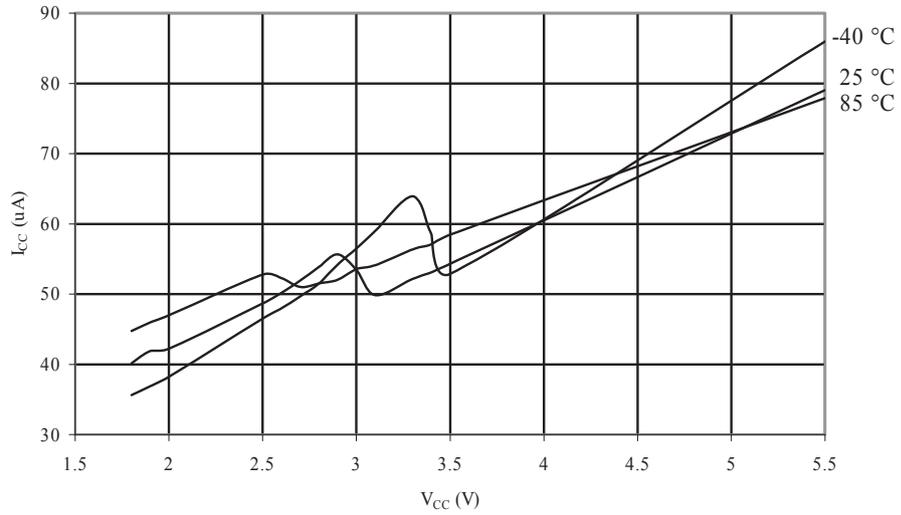
**Figure 34-136. ATmega168A: AREF External Reference Current vs. V<sub>CC</sub>**
