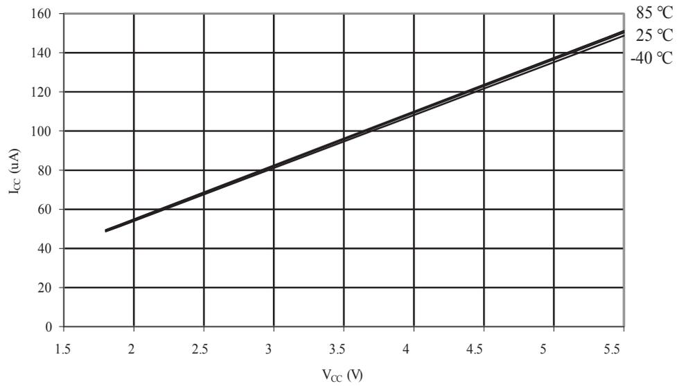
Figure 34-90. ATmega88A: Brownout Detector Current vs.  $V_{CC}$
