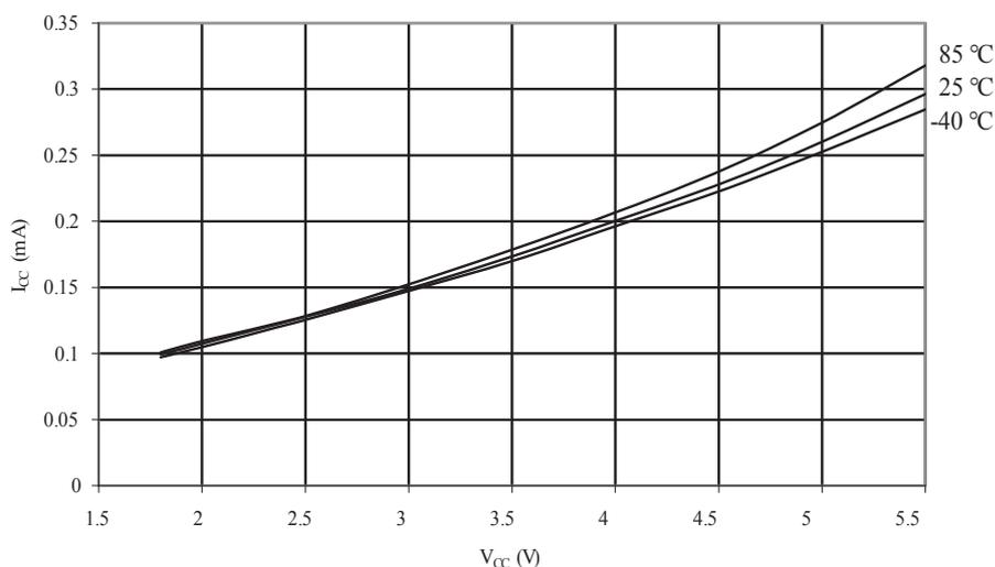
**Figure 34-57. ATmega88A: Idle Supply Current vs. V<sub>CC</sub> (Internal RC Oscillator, 8MHz)**
