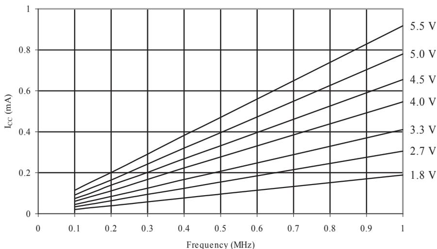
**Figure 34-2. ATmega48A: Active Supply Current vs. Frequency (1MHz - 20MHz)**
