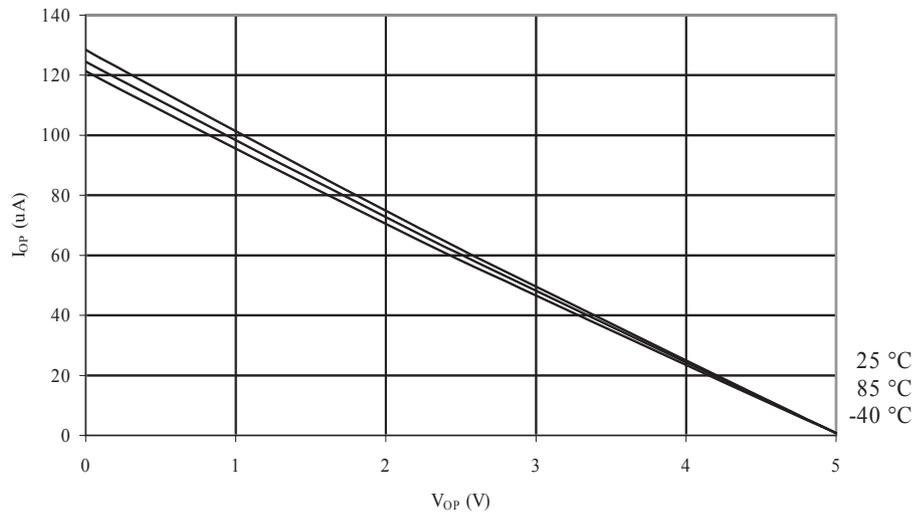
**Figure 34-18. ATmega48A: Reset Pull-up Resistor Current vs. Reset Pin Voltage ( $V_{CC} = 1.8V$ )**
