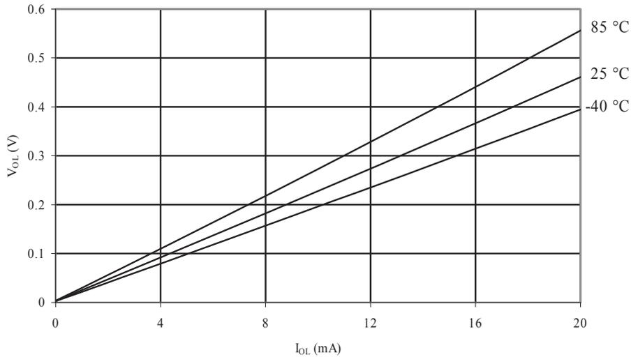
Figure 34-117. ATmega168A: I/O Pin Output Voltage vs. Source Current ( $V_{CC} = 3V$ )
