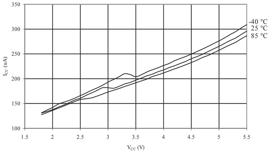
**Figure 34-135. ATmega168A: Analog Comparator Current vs. V<sub>CC</sub>**
