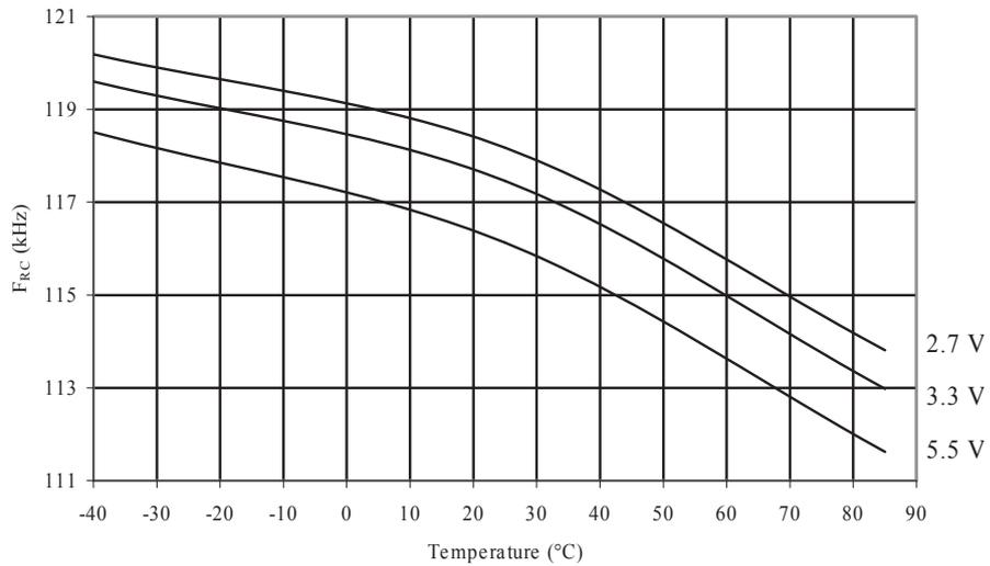
**Figure 34-130. ATmega168A: Watchdog Oscillator Frequency vs.  $V_{CC}$**
