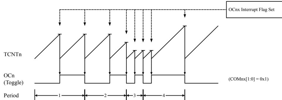
An interrupt can be generated each time the counter value reaches the TOP value by setting the OCF0A Flag. If the interrupt is enabled, the interrupt handler routine can be used for updating the TOP value.
