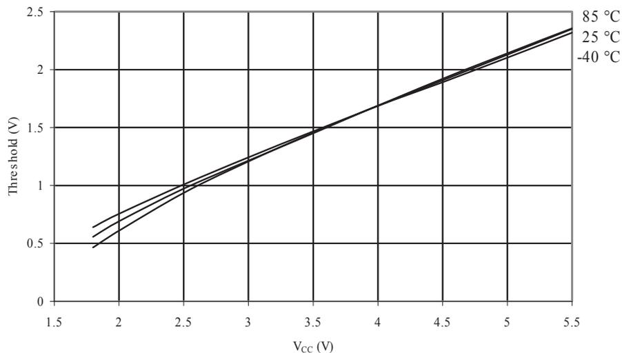
Figure 34-27. ATmega48A: I/O Pin Input Hysteresis vs.  $V_{CC}$
