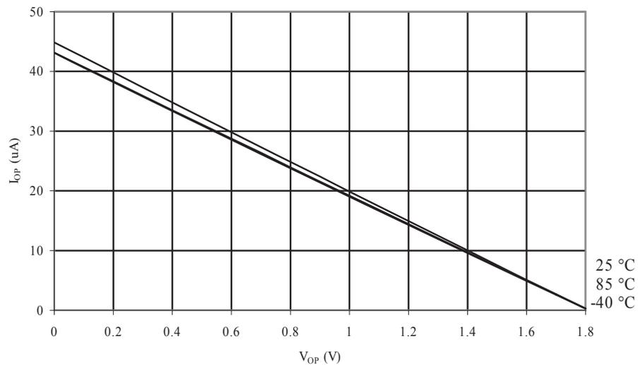
**Figure 34-16. ATmega48A: I/O Pin Pull-up Resistor Current vs. Input Voltage ( $V_{CC} = 2.7V$ )**
