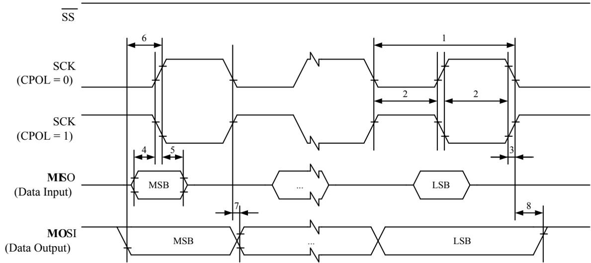
**Figure 33-4. SPI Interface Timing Requirements (Slave Mode)**
