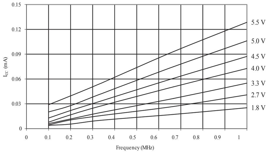
Figure 34-54. ATmega88A: Idle Supply Current vs. Frequency (1-20MHz)
