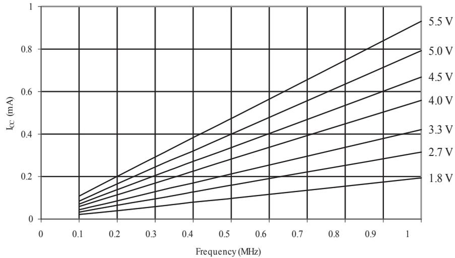
Figure 34-49. ATmega88A: Active Supply Current vs. Frequency (1 - 20MHz)
