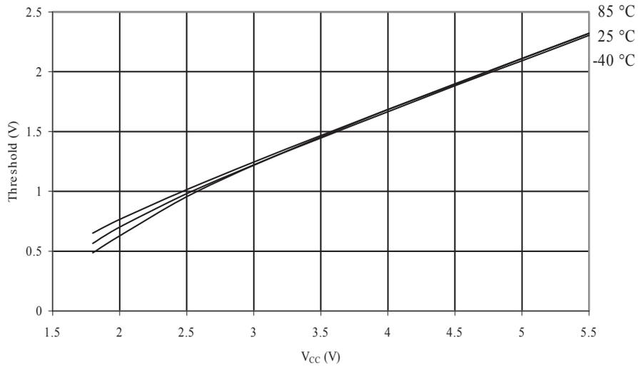
**Figure 34-121. ATmega168A: I/O Pin Input Hysteresis vs.  $V_{CC}$**
