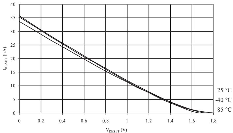
Figure 34-113. ATmega168A: Reset Pull-up Resistor Current vs. Reset Pin Voltage ( $V_{CC} = 2.7V$ )
