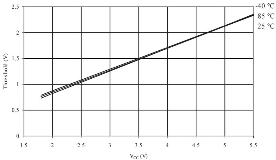
**Figure 34-124. ATmega168A: Reset Pin Input Hysteresis vs.  $V_{CC}$**
