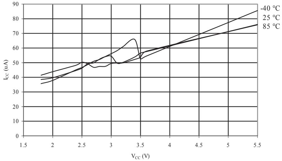
Figure 34-42. ATmega48A: AREF External Reference Current vs. V<sub>CC</sub>
