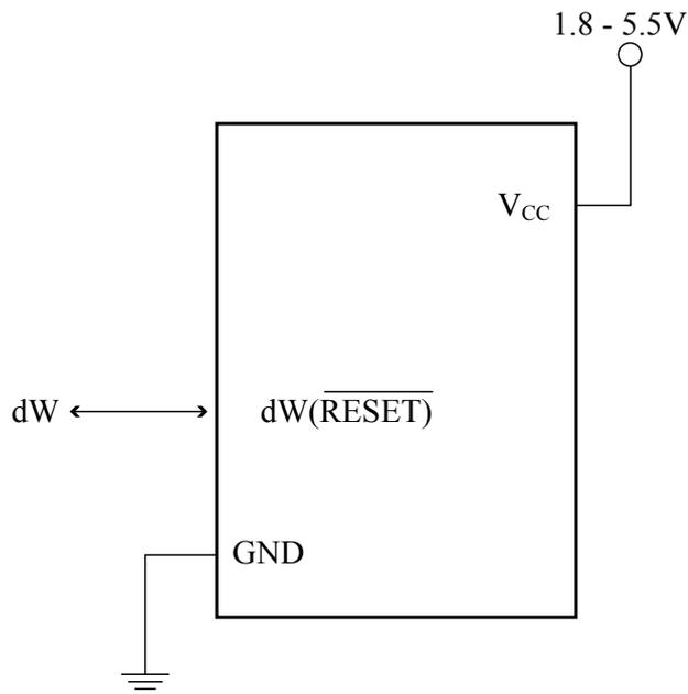
Figure. The debugWIRE Setup shows the schematic of a target MCU, with debugWIRE enabled, and the emulator connector. The system clock is not affected by debugWIRE and will always be the clock source selected by the CKSEL Fuses.
