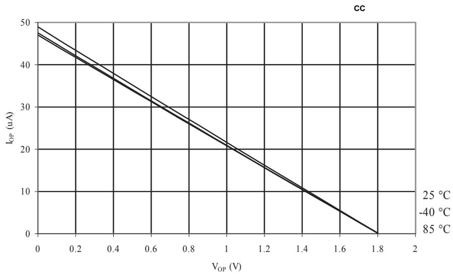
**Figure 34-110. ATmega168A: I/O Pin Pull-up Resistor Current vs. Input Voltage ( $V_{CC} = 2.7V$ )**
