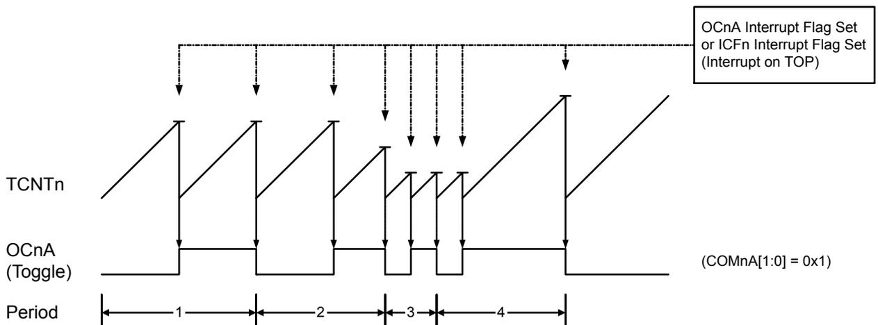
**Note:** The “n” in the register and bit names indicates the device number ( $n = 1$  for Timer/Counter 1), and the “x” indicates Output Compare unit (A/B).
