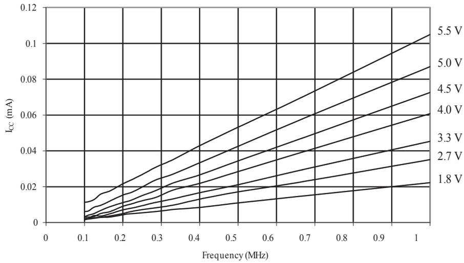
Figure 34-93. ATmega88A: Reset Supply Current vs. Frequency (1 - 20MHz)
